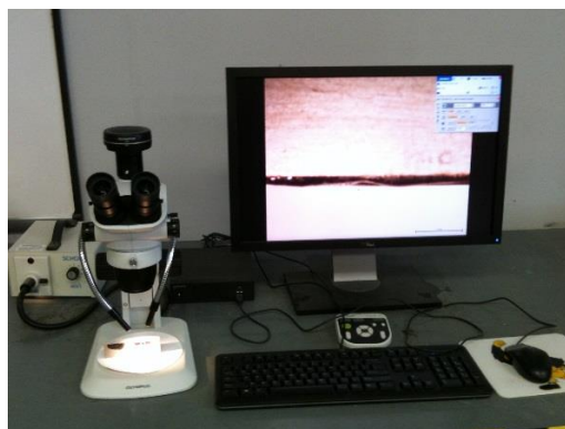
Figure 4.13 Asphalt Sample &amp; Aggregate Plate Cross-sectional Cut under the Microscope
