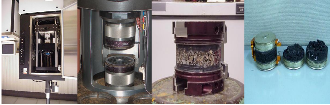
Figure 2.14 Superpave Shear Tester, Loading Chamber, Prepared Sample, and Samples after Test (12).
