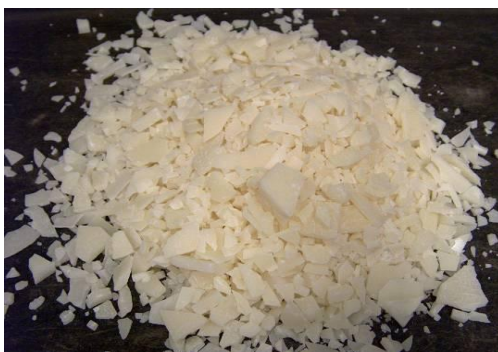
Figure 2.28 LEADCAP Warm Mix Asphalt Additive (38).
