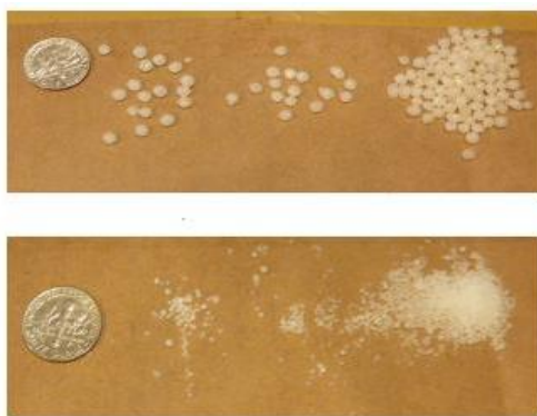
Figure 2.27 Sasobit Pastille (ca 4 mm diameter) & Prill (ca 1 mm diameter) Forms (37).
