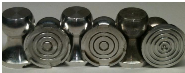
Figure 4.11 0.8 mm (left), 0.4 mm (middle) and 0.0 mm (right) Pullout Stubs.
