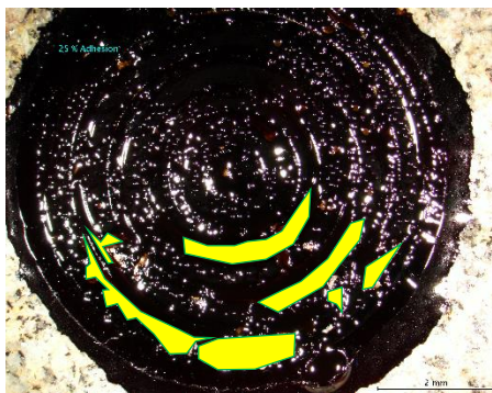
Figure 4.15 Test Sample with 75% Cohesive Failure.
