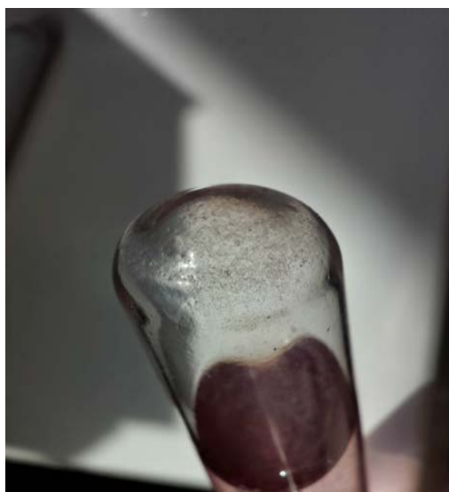
Figure A-8: Bottom of 10 mg/L test tube from Experiment 3. The unaccounted for Au is expected to have accumulated at the bottom of the test tube or sorbed to the glassware.
