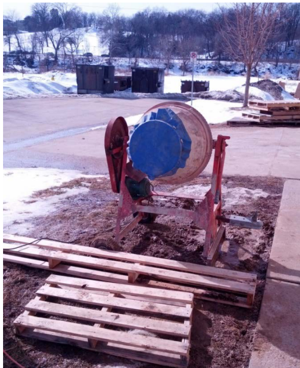
Figure 3.4. Concrete mixer (along with two heavy bricks) used to pulverize sediment from field site.
