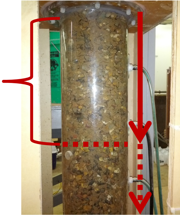
Figure 4.18. Visible intrusion of sediment from the surface at the end of Run A4. The maximum infiltration depth of fine sediments into a stable gravel bed has been reported to be between 10 and 30 cm (Beschta and Jackson, 1979; Diplas and Parker, 1984).
