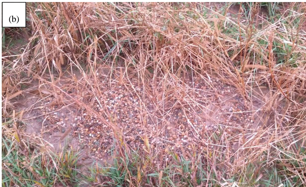
Figure 2.9. (a) ATI surface (July 2013); (b) further silted and vegetated over ATI surface (October 2013).
