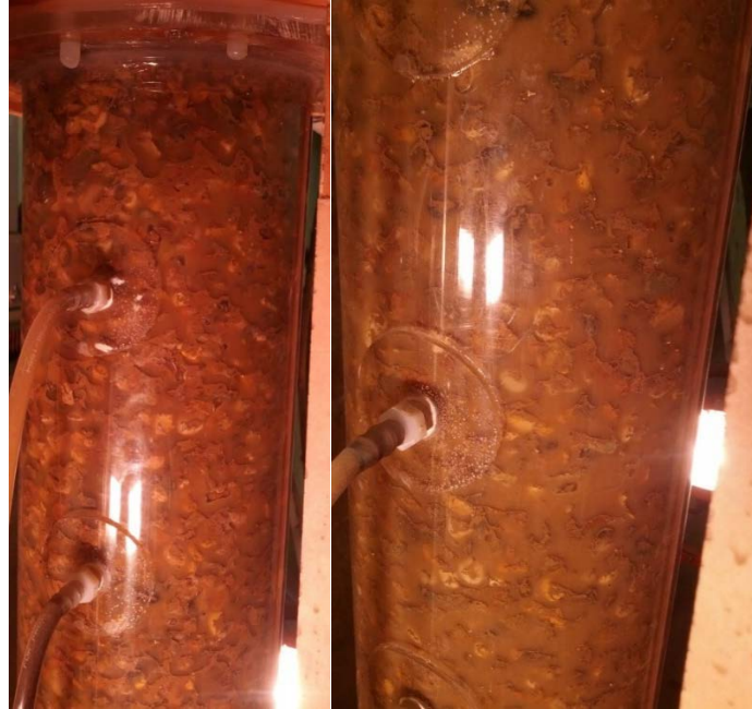
Figure 4.19. Observed bridging of sediment across grains of pea gravel in the permeameter.
