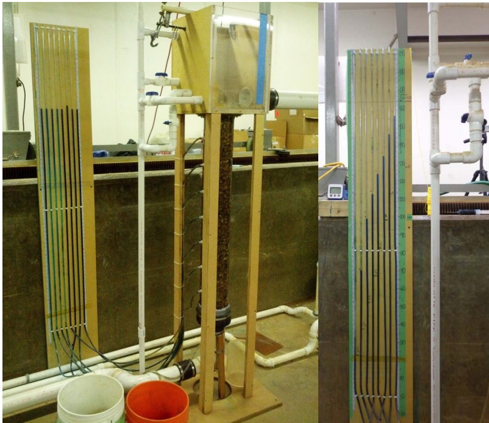
Figure 3.1. The (a) permeameter (clear acrylic tube) complete with eight pressure taps and manometer under hydrostatic pressure; and (b) with water flowing.
