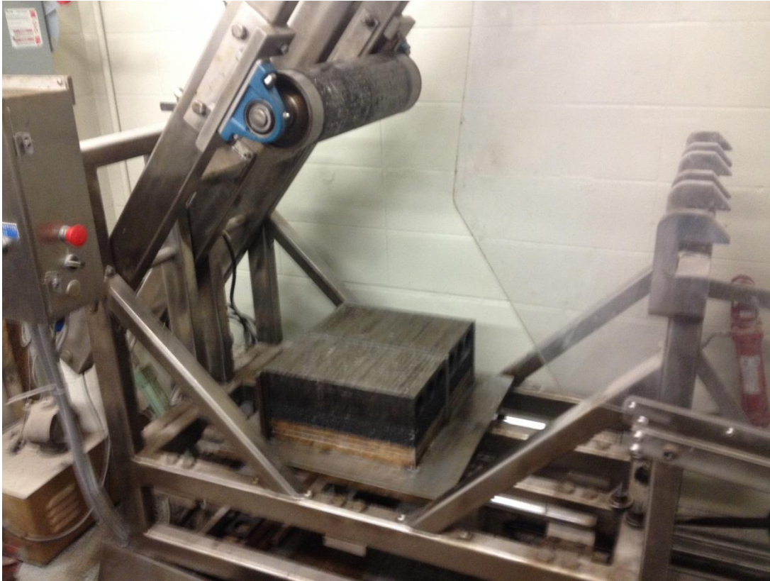
Figure 3-2. Resulting Compacted slab
