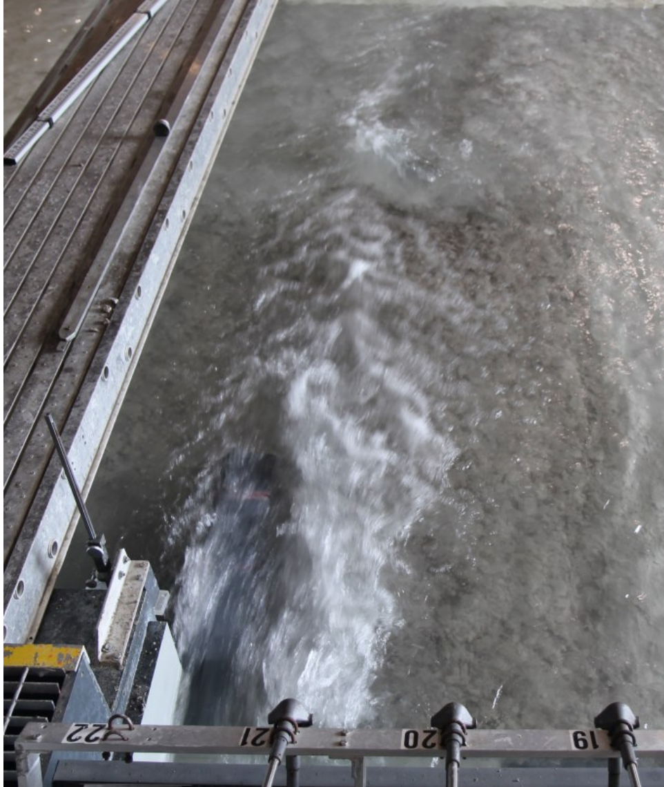
Figure 3-9. Full open gate 22 scour test underway
