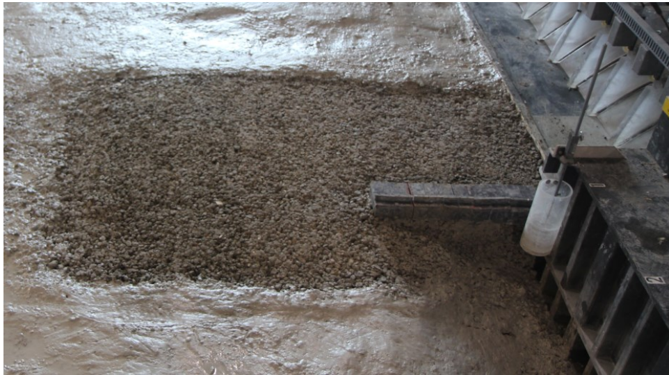
Figure 3-8. Photographs of the initial bathymetry and segmented training wall for the spillbay 22 full open gate scour test
