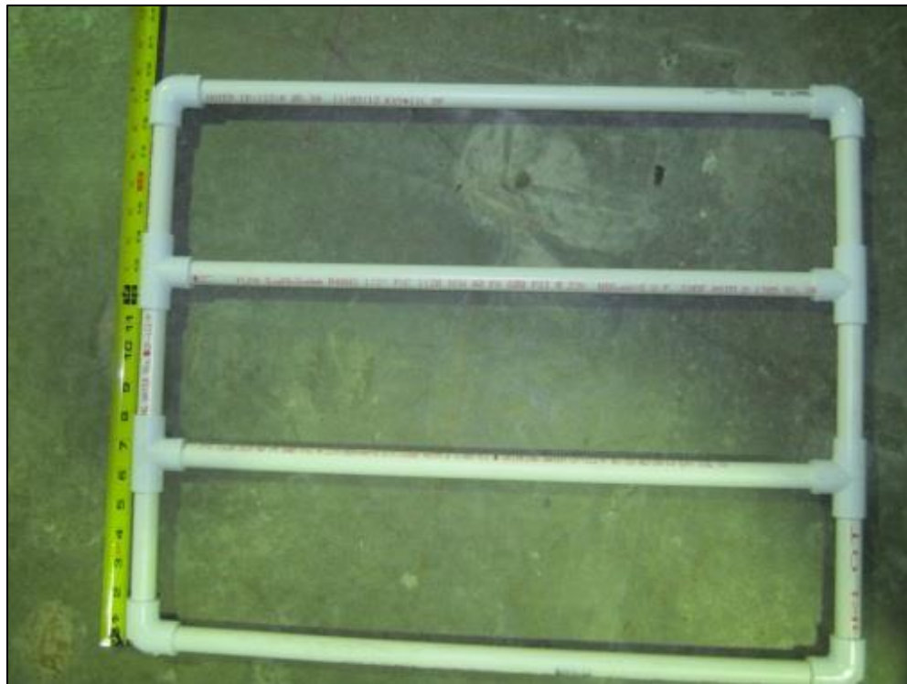
Figure A8. An image of the aeration distribution system (with dimensions) prior to perforations.
