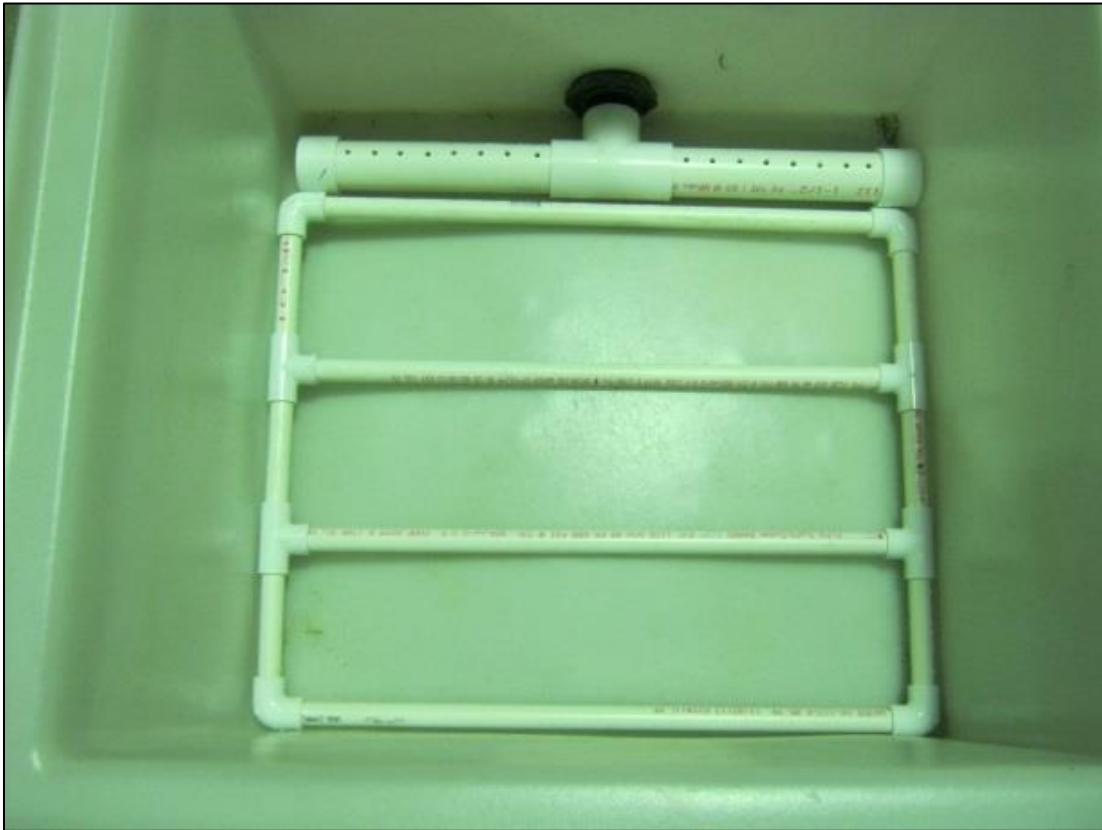
Figure A6. An image of the effluent manifold (perforated PVC penetrating the wall of the container).
