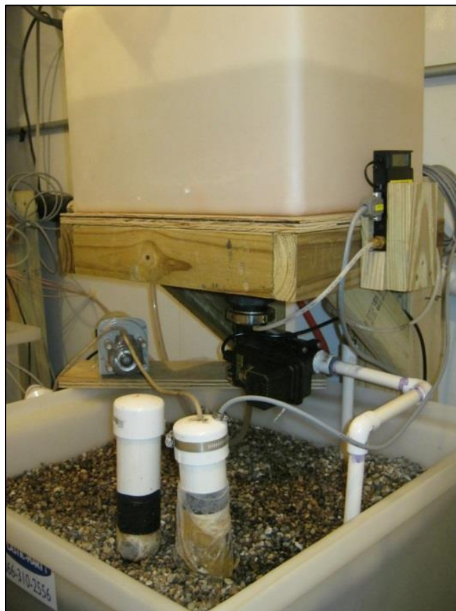
Figure A14. An image of SAGB4, equipped with pH-controlled aeration and recirculation.
