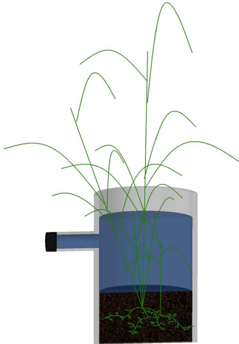
Figure 2-13: Control with plants, non-contaminated soil, and no oil slick. The bottom, brown phase is normal sediment, the clear blue phase is the water and the green is Spartina alterniflora .
