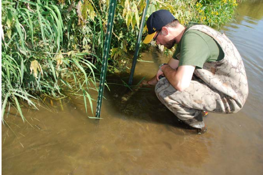
Figure 3.3 Deployment of PSFM at the Oxford site. The sampler is placed on the downstream post with the upstream post acting as a debris shield. Picture courtesy of Sarani Rangarajan.
