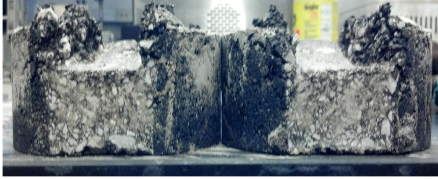
Figure 3.39: Test LW3 (64-22) specimens after testing
