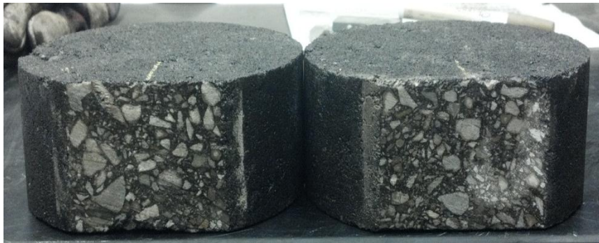
Figure 4.17: Test FH2 specimens before testing (side)
