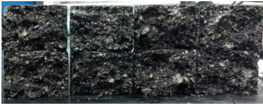
Figure 3.14: Stripping effects on lab mixed WMA specimens
