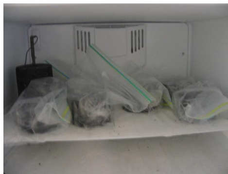
Figure A9: Freezing of the wet specimens at -18^{\circ}\text{C} for 16 hours
