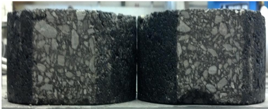
Figure 3.25: Test LW2 (PG 58-28) specimens before testing (side)
