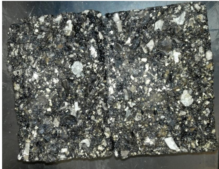
Figure 5.2: Stripping on a lab mixed WMA specimen
