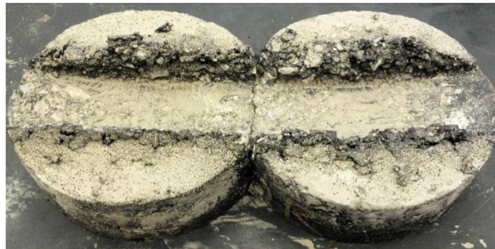
Figure 3.38: Test LW3 (64-22) specimens after testing
