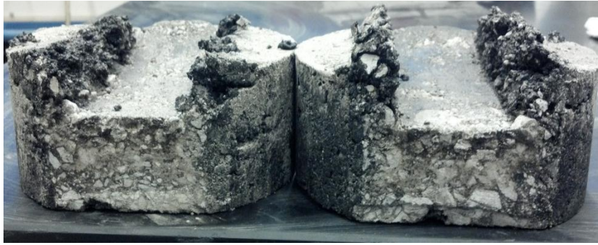
Figure 3.21: Test LH1 (PG 58-28) specimens after testing (side)
