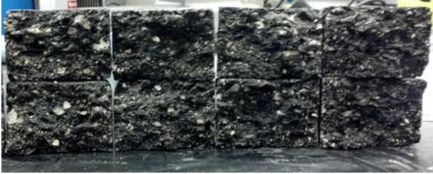
Figure 3.13: Stripping effects on lab mixed HMA specimens
