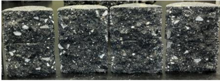
Figure 4.12: Stripping effects on field mixed HMA specimens
