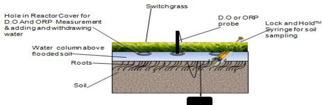
**Figure A10: Schematic of reactor used in experiment with soil from Amana colonies and that had cycling of moisture content and redox potential. Samples were collected using a Lock and Hold syringe to make a vertical core in the soil column. D.O and ORP measurements were taken by inserting the probe through a 1.9 cm hole drilled in the cover of the reactor. The switchgrass planted system is used as an example.**
