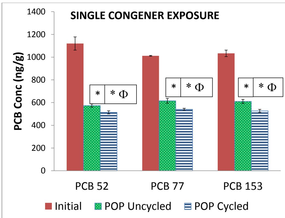
**Figure 3.7: Dissipation of PCB in soil contaminated with PCB 52, PCB 77 and PCB 153 as the sole contaminants and planted with poplar. POP = poplar. The spiked congeners were undetectable in the controls which were not spiked. \*= significant reduction when compared to initial concentration ( $p < 0.05$ ).  $\Phi$  = significantly higher reduction when compared to uncycled treatment ( $p < 0.05$ ). Error bars are 1 standard deviation and  $n=3$ .**
