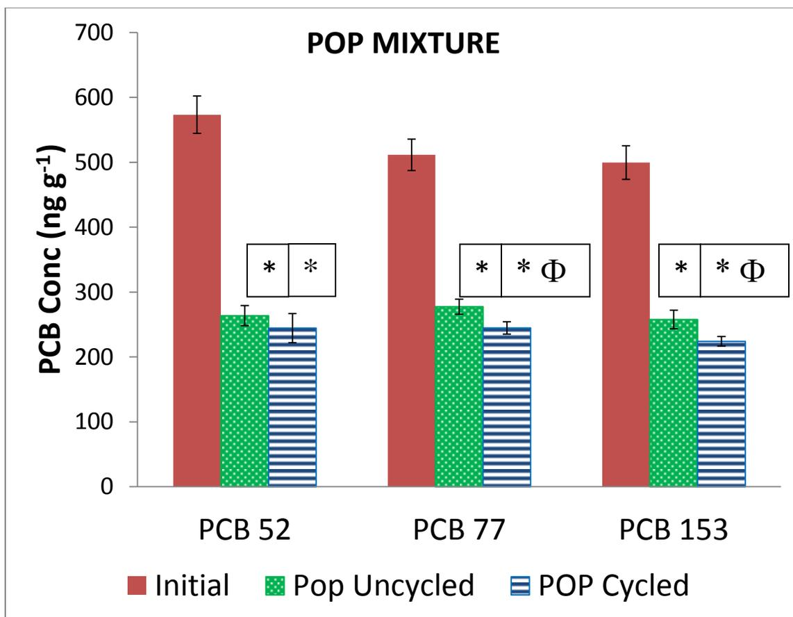
**Figure 3.6: Dissipation of PCB in soil contaminated with mixture of PCB 52, PCB 77 and PCB 153 and planted with poplar. POP = Poplar. The spike congeners were undetectable in the controls which were not spiked. \*= significant reduction when compared to initial concentration ( $p < 0.05$ ).  $\Phi$  = significantly higher reduction when compared to uncycled treatment ( $p < 0.05$ ). Error bars are 1 standard deviation and  $n=3$ .**
