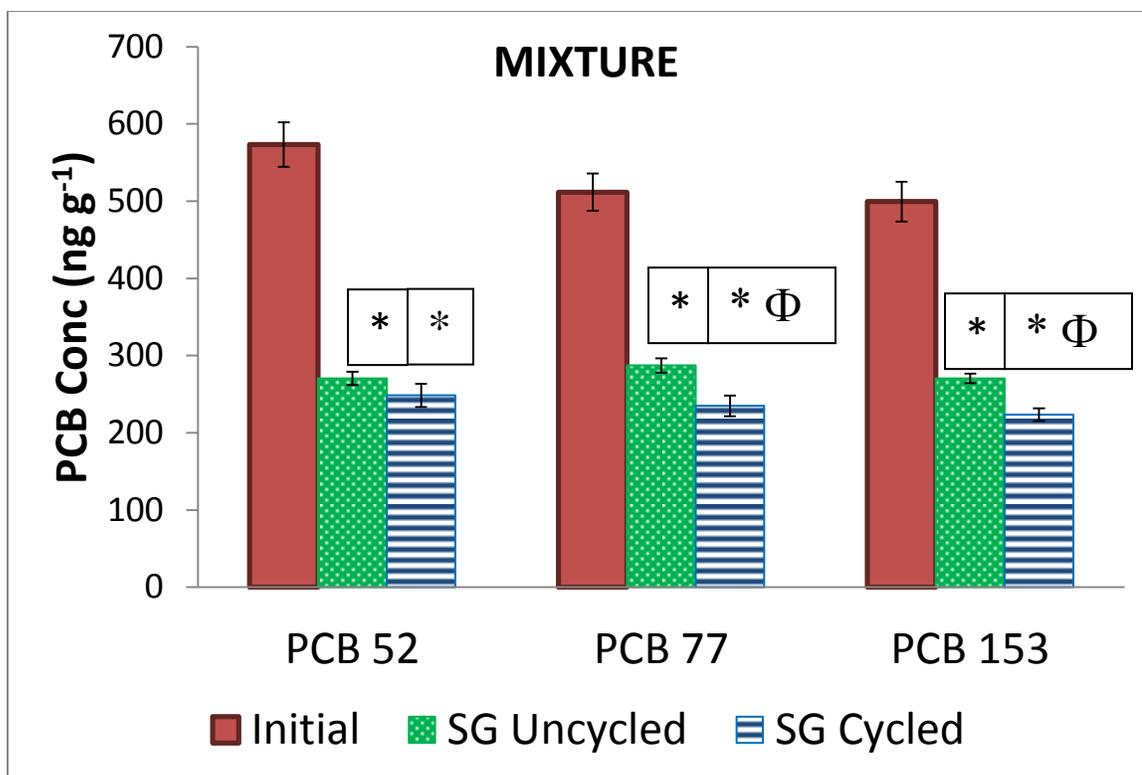
**Figure 3.4: Dissipation of PCB in soil contaminated with mixture of PCB 52, PCB 77 and PCB 153 and planted with switchgrass. SG = switchgrass. The spike congeners were undetectable in the controls which were not spiked. \*= significant reduction when compared to initial concentration ( $p < 0.05$ ).  $\Phi$  = significantly higher reduction when compared to uncycled treatment ( $p < 0.05$ ). Error bars are 1 standard deviation and  $n=3$ .**
