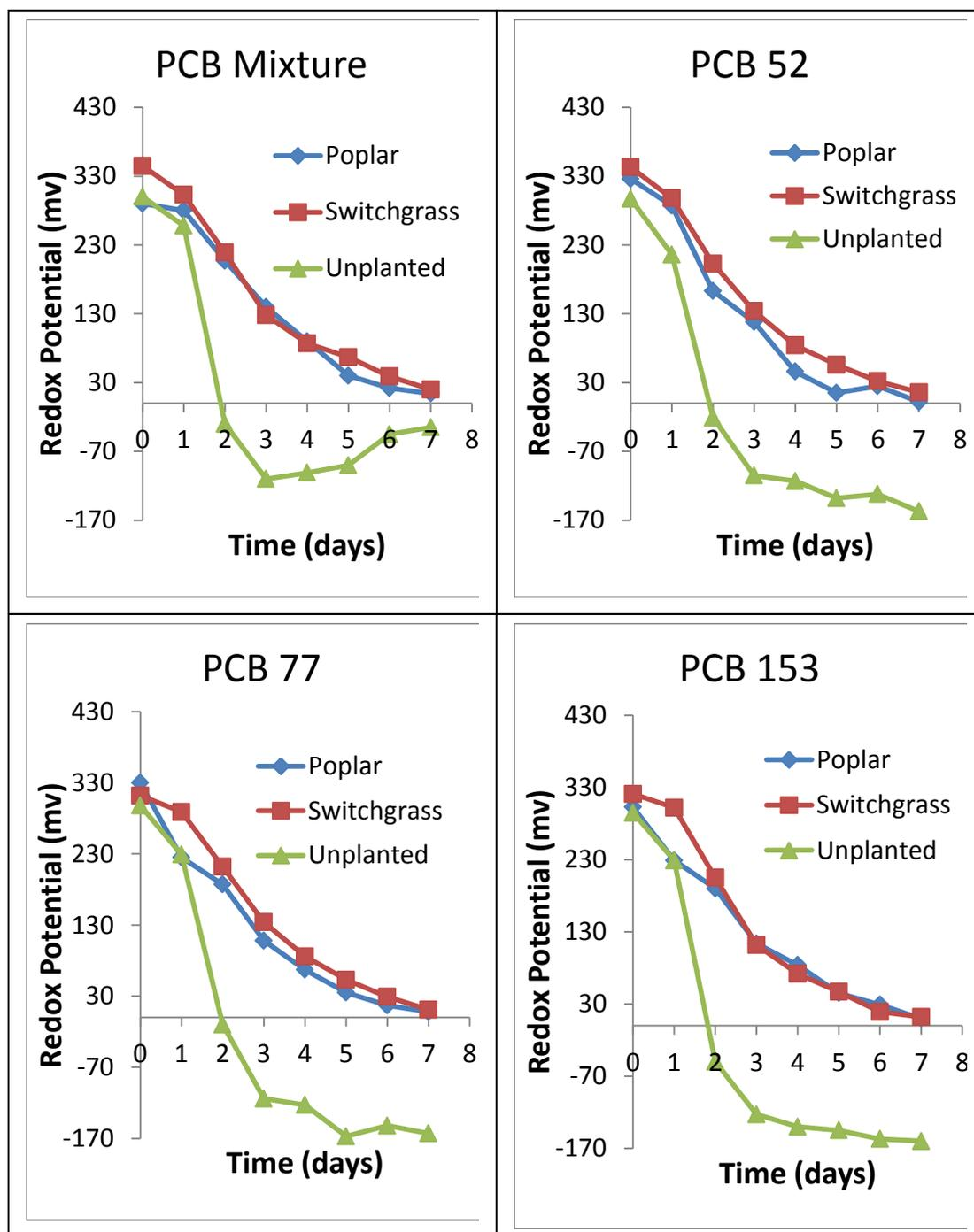
**Figure 3.2: Representative redox potential in flooded soil containing a mixture of PCB 52, 77 and 153 and single congeners and planted with switchgrass or poplar. Also shown is the redox potential in the flooded unplanted system.**
