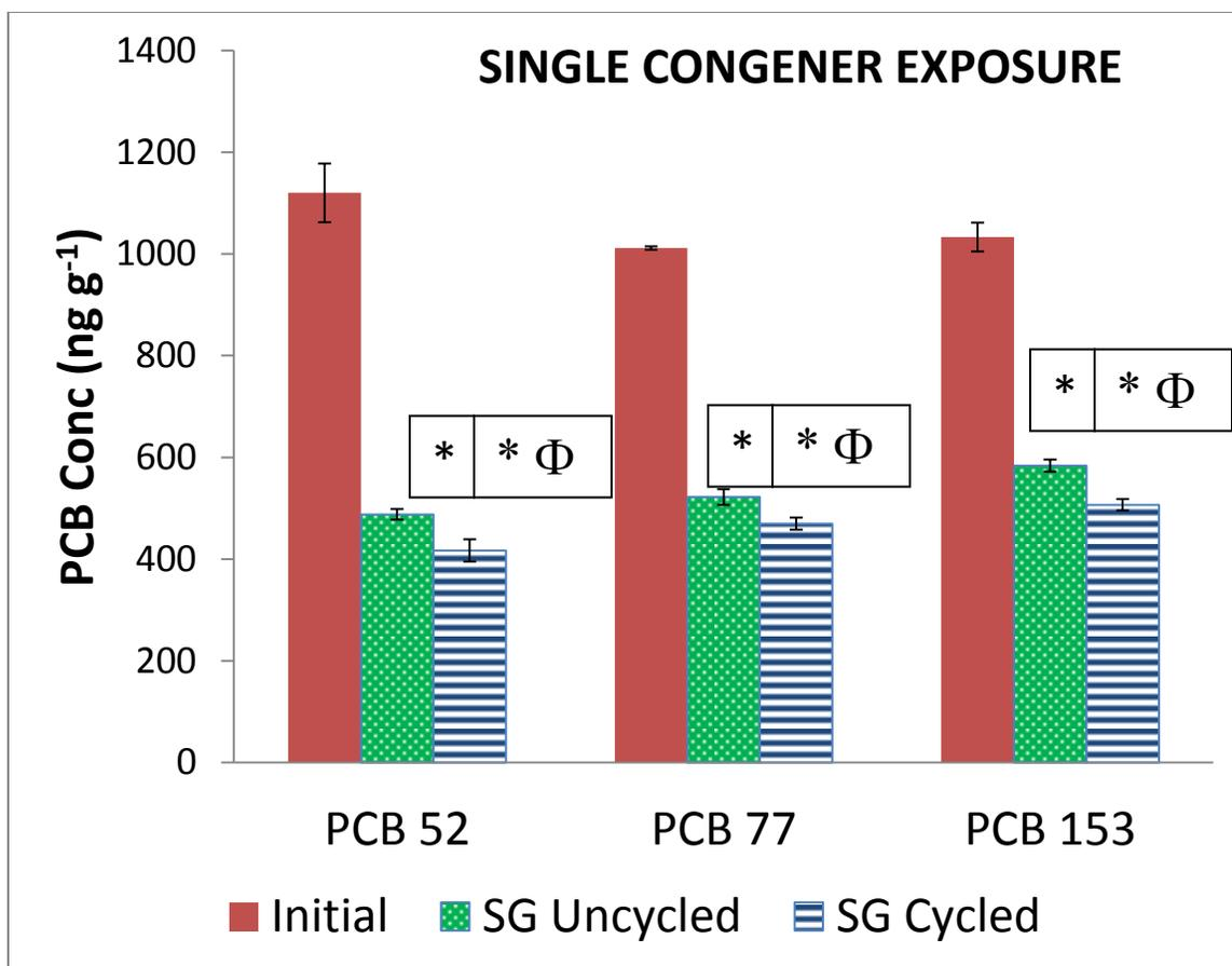
**Figure 3.5: Dissipation of PCB in soil contaminated PCB 52, PCB 77 and PCB 153 as the sole contaminants and planted with switchgrass. SG = switchgrass. The spiked congeners were undetectable in the controls which were not spiked. \* = significant reduction when compared to initial concentration ( $p < 0.05$ ).  $\Phi$  = significantly higher reduction when compared to uncycled treatment ( $p < 0.05$ ). Error bars are 1 standard deviation and  $n=3$**
