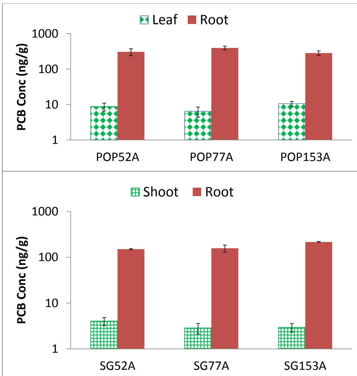
**Figure 4.8: Distribution of parent compounds in plant material after 32 weeks of planting in PCB contaminated soil. Top chart is poplar; bottom chart is switchgrass. Error bars are 1 standard deviation and are based on triplicate measurements.**
