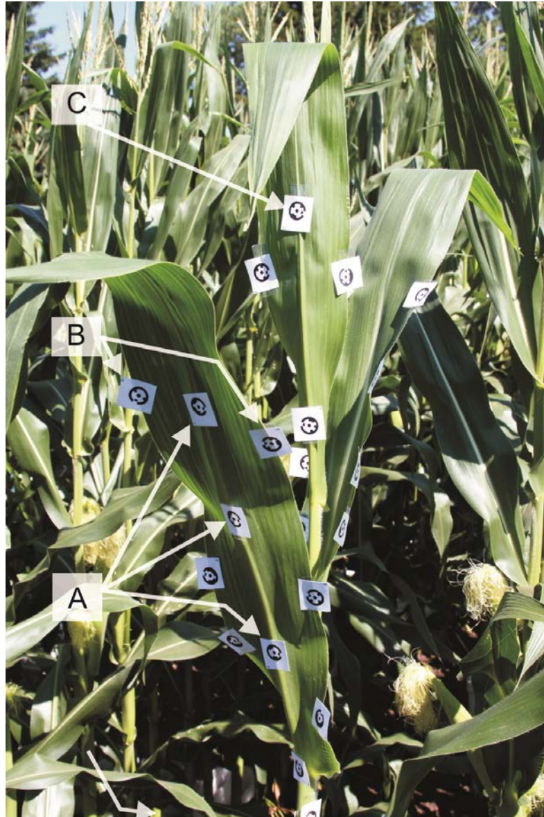
Figure V-3. Leaf ready for image acquisition. (A) points to the mid-rib of the leaf that is currently being digitized, (B) indicates targets on the edges of the leaf and (C) points to targets on other leaves that are used to combine individual leaf models (cross-referencing points). Photography used in the digitizing of the leaves on 13 July 2010.
