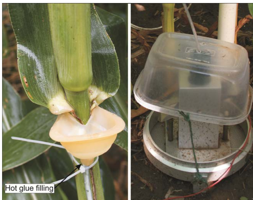
Figure III-1. The left hand side shows a view of the stemflow collector attached to the maize stem. The right hand side shows the modified tipping bucket with indirect rainfall protection. Tubing is attached to a stemflow collector that redirects the water flowing down the stem to the tipping bucket gauge.
