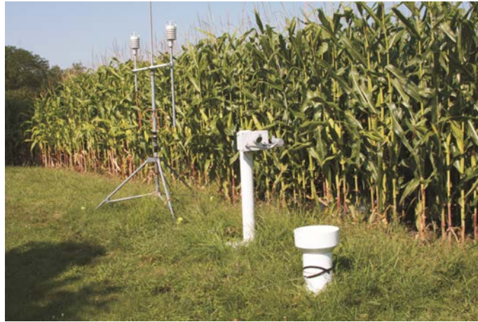
Figure III-5. Instrumentation installed outside of the canopy, including one tipping bucket rain gauge, one optical disdrometer, and two compact weather stations.
