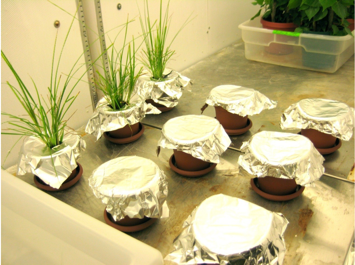
Figure 2-1. The experimental setup for the RDX microcosm study. Includes three replicates planted in soil from Eglin Air Force Base with Bahiagrass Pensacola, three with excised Bahiagrass Pensacola roots, and three unplanted. All replicates were covered with aluminum foil. Not shown: the poplar and excised poplar root microcosms.
