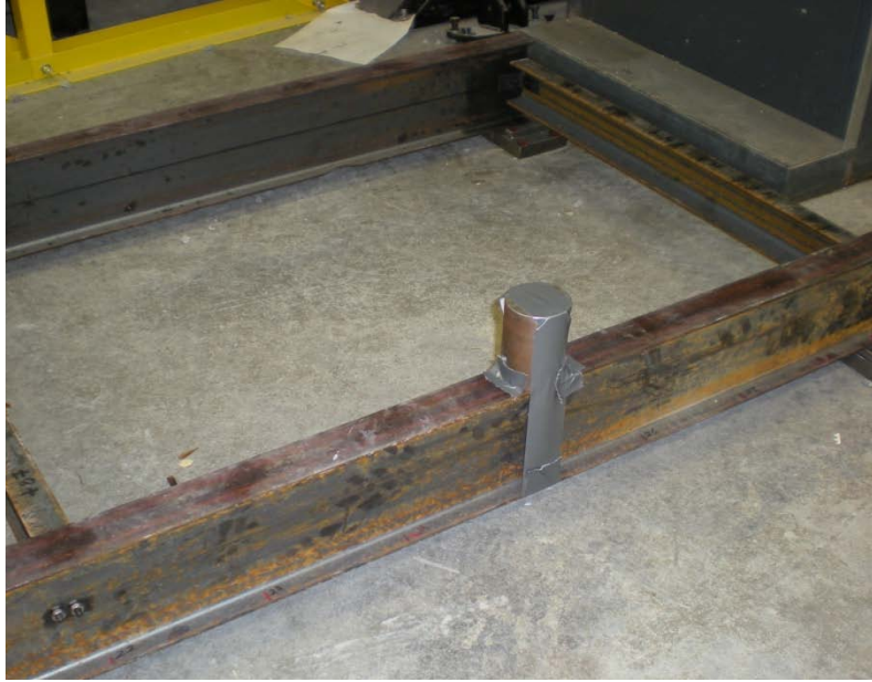
Figure 3.27 Mass (1500 g) added to top flange of the right beam, 20 inches from the far end
