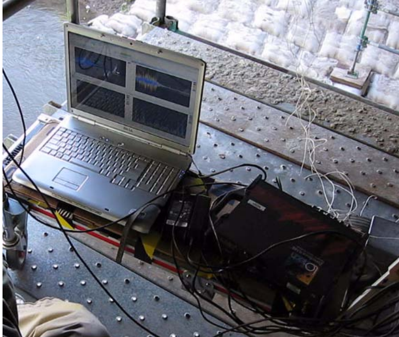
Figure 4.3 Typical field operational vibration test setup
