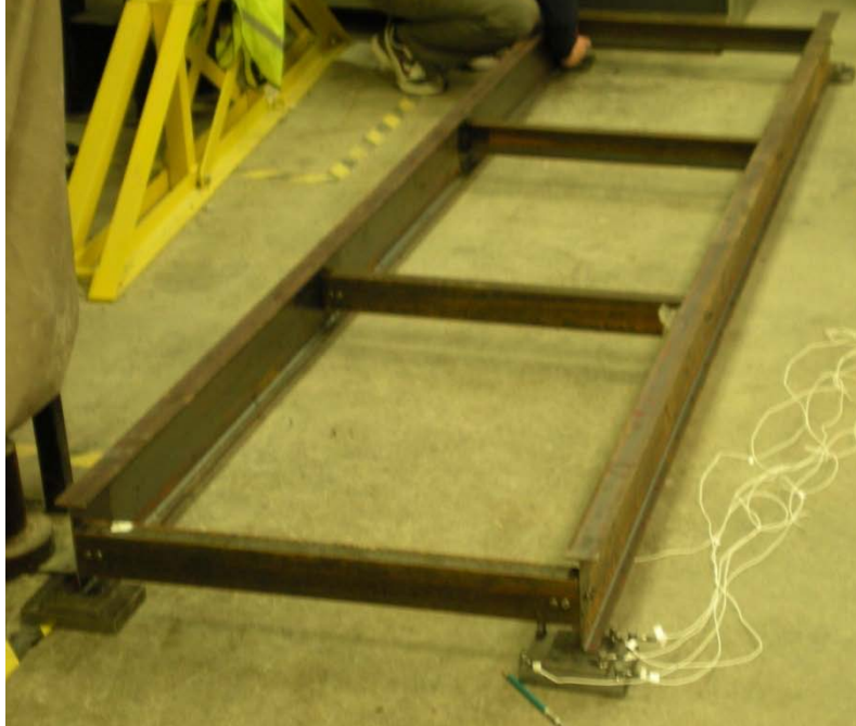
Figure 3.21 Scale bridge in the laboratory
