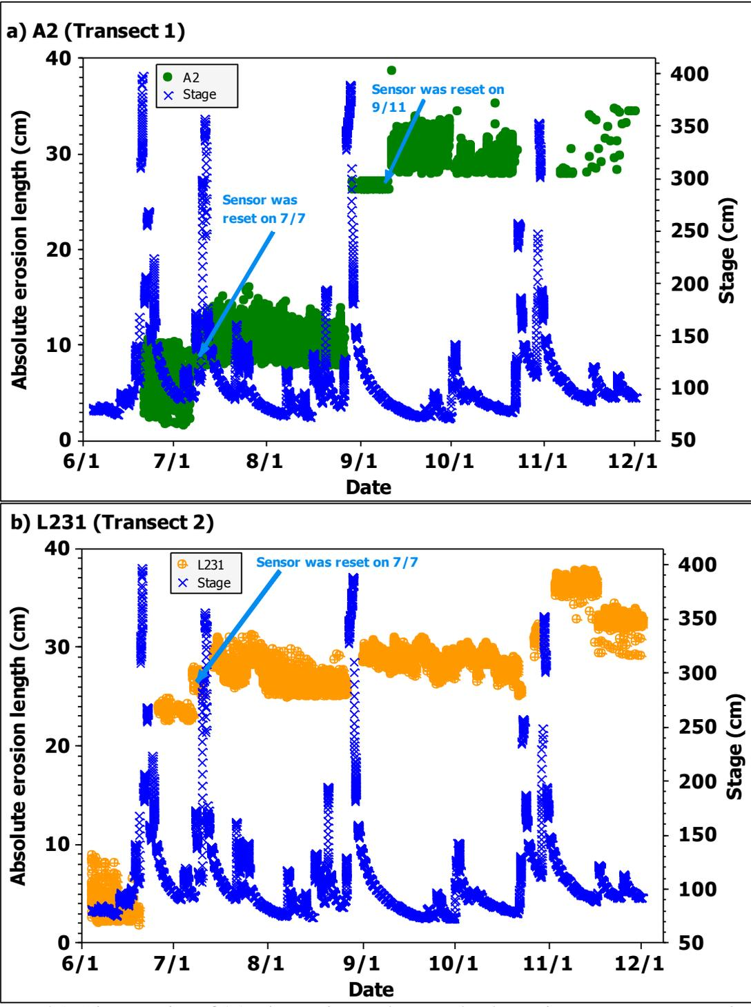
Figure 4.9: Times series of 15-minutes interval, stage, bank erosion measurements using the sensors at Camp Cardinal (Site 2)
