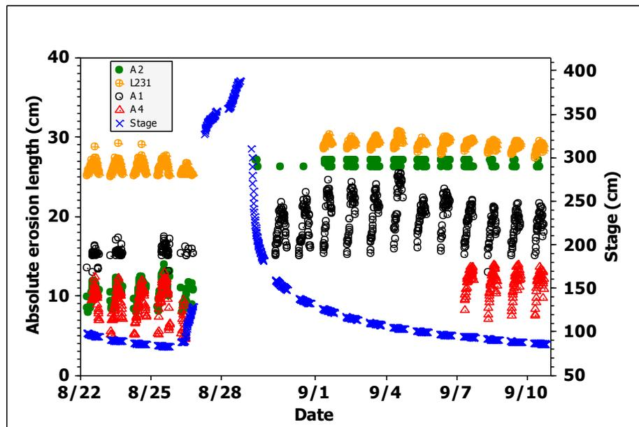
Figure 4.12: Erosion measurements at an event scale before, during and after the high flow event of August 27<sup>th</sup> at Camp Cardinal. The x-axis is the 15-minutes interval, the primary y-axis is the erosion measurements in cm and the secondary y-axis is the water stage in cm.
