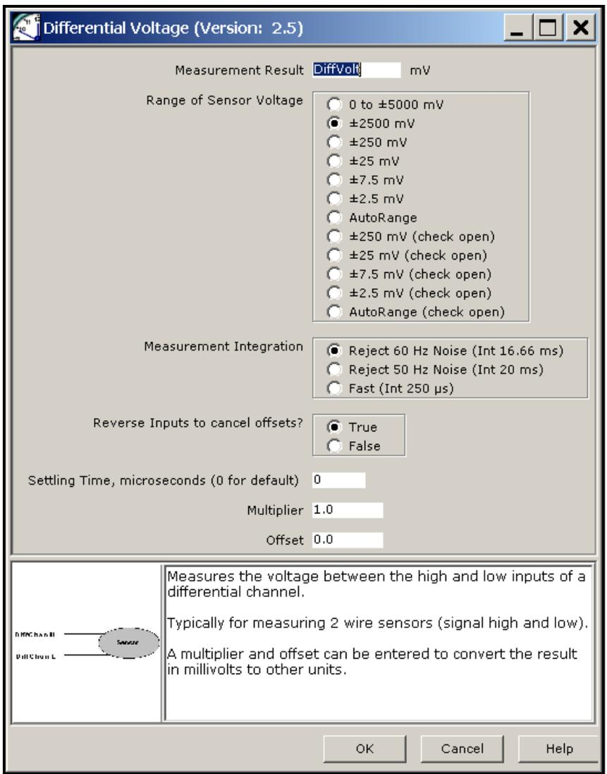
Figure A.2: Specifications of the program PEEP\_01
