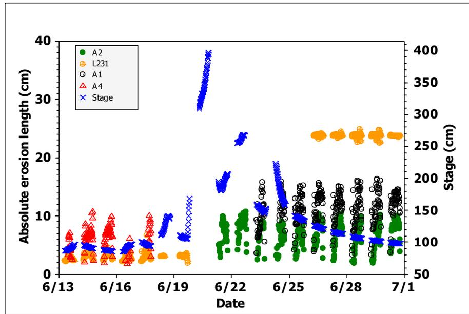
Figure 4.11: Erosion event-based measurement before, during and after the June 19<sup>th</sup> storm event at Camp Cardinal. The x-axis is the 15-minutes interval, the primary y-axis is the absolute erosion measurements in cm and the secondary y-axis is the water stage in cm.
