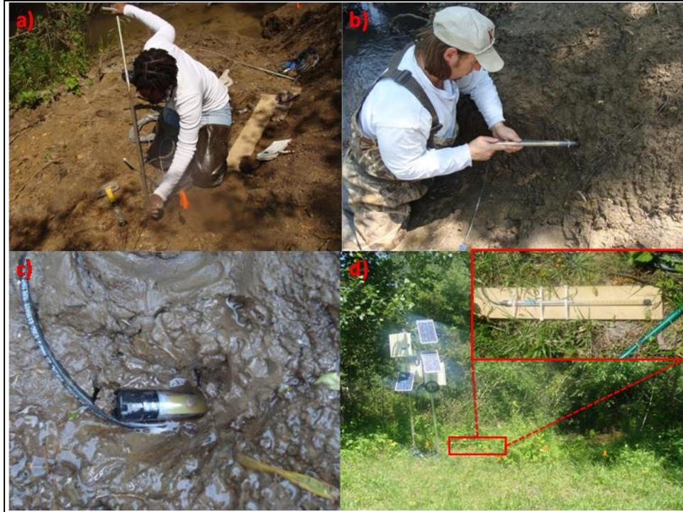
Figure 3.13: Installation procedure for the PEEPs.
