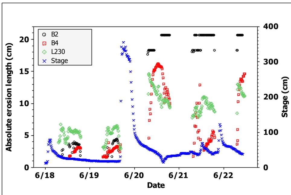
Figure 4.2: Erosion event-based measurement before, during and after the June 19<sup>th</sup> storm event at South Amana. The x-axis is the 15-minute interval, the primary y-axis is the absolute erosion measurements in cm and the secondary y-axis is the water stage in cm.
