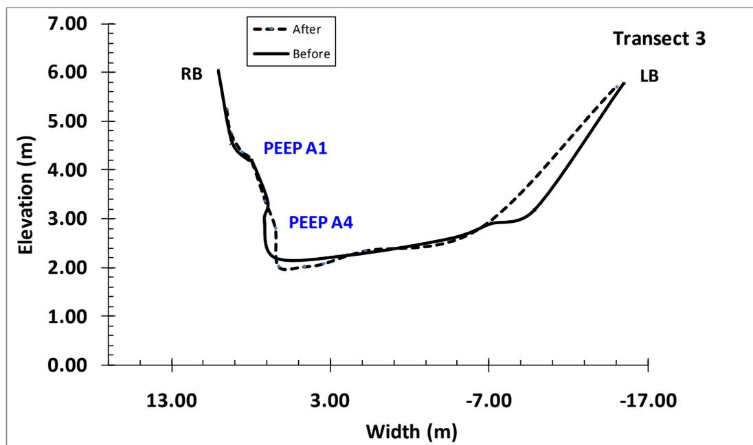
Figure 4.14: Delimitation of the PEEP transect 3 before and after the August 27<sup>th</sup> event. The bank profile is delimited using the survey data of July 30<sup>th</sup> and September 30<sup>th</sup> 2009. Facing downstream, “RB” stands for Right bank and “LB” for left bank.
