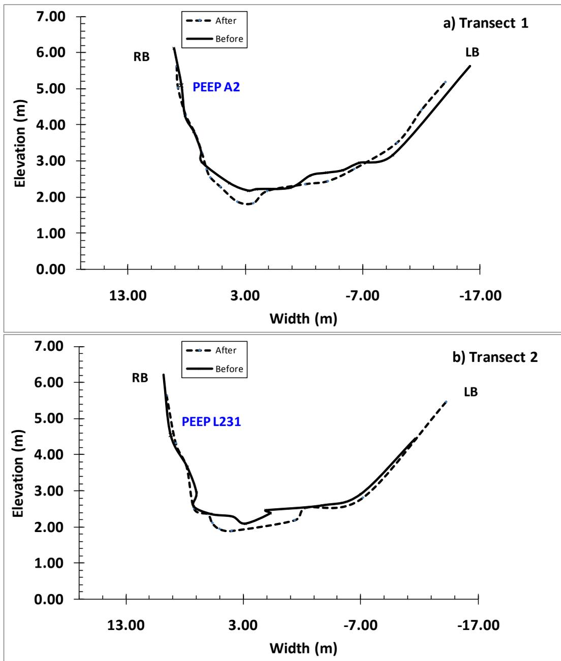
Figure 4.13: Delimitation of the PEEP transects before and after the August 27<sup>th</sup> event. The bank profile is delimited using the survey data of July 30<sup>th</sup> and September 30<sup>th</sup> 2009. Facing downstream, “RB” stands for Right bank and “LB” for left bank.
