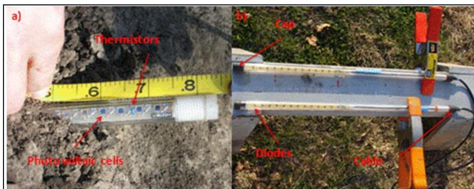
Figure 3.9: Picture of the PEEP sensors.
