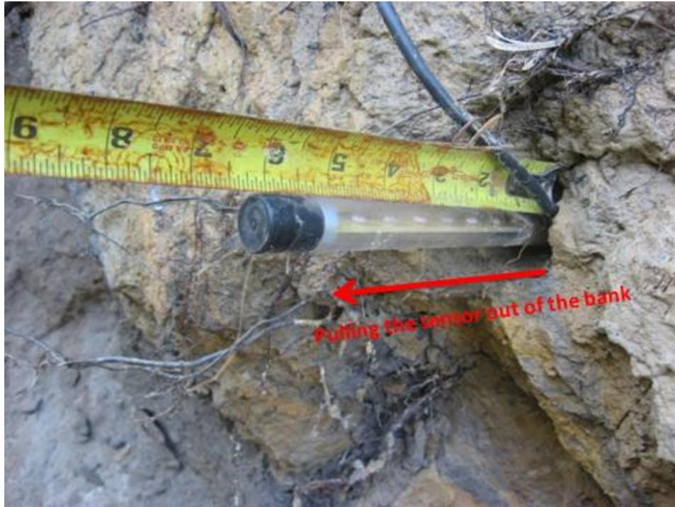
Figure 3.11: In-bank calibration of the PEEP.
