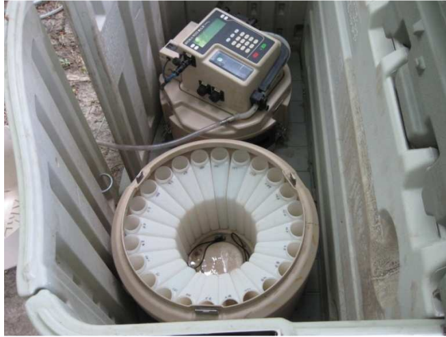
Figure 4.3. Sigma sampler: the computer and pump are displayed in the top of the picture while the bottles used to store the samples are on the bottom
