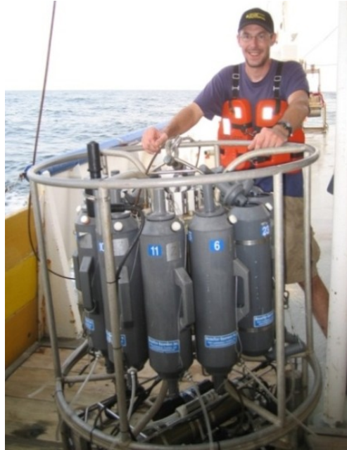
Figure 2-6. Aaron Gwinnup onboard the R/V Pelican, with the "CTD" array which is deployed to measure multiple water quality parameters simultaneously, as well as take grab samples of the water column at various depths with a rosette of "Niskin" bottles
