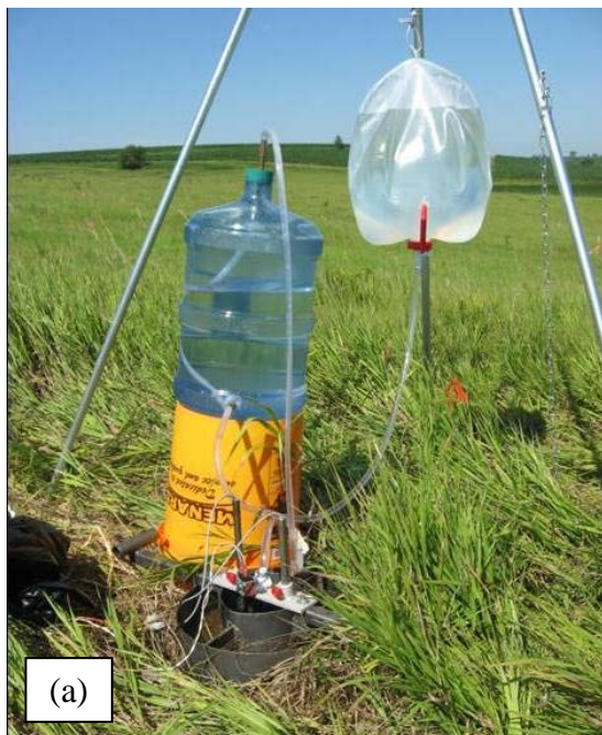
Figure 3.4 The University of Iowa Double Ring Infiltrometer: (a) general view of the setup; (b) close view of the sensors.
