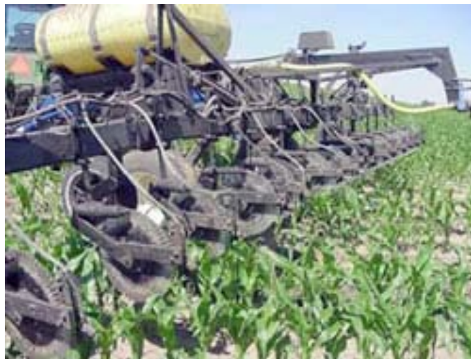
Figure 1.1. A typical liquid-N toolbar used in Iowa to side dress corn in early summer. http://www.yetterco.com
