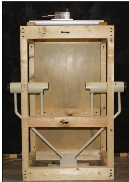
Figure 21 – Steel Sphere Experimental Setup. The steel spheres were dropped from a height of 0.396 meters.
