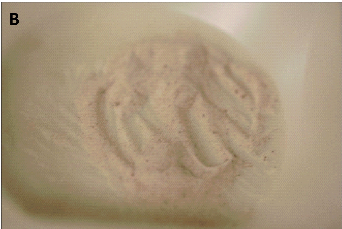
Figure 3.1: Zoledronic acid (A) after mixing with food coloring and (B) after further mixing into PMMA.
