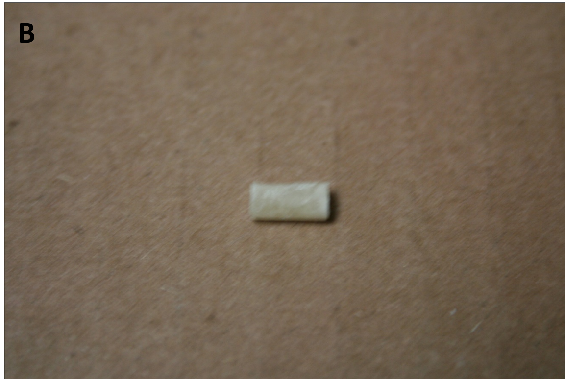
Figure 3.2: Sample PMMA cylinder (A) after removal from mold and (B) after trimming prior to compression.
