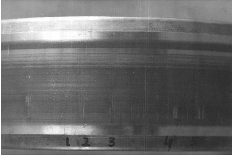
Fig. 4.9. Inner race of bearing NU 326 on exposure of 50 A (AC) for 250 h (using lubricant 'A')
