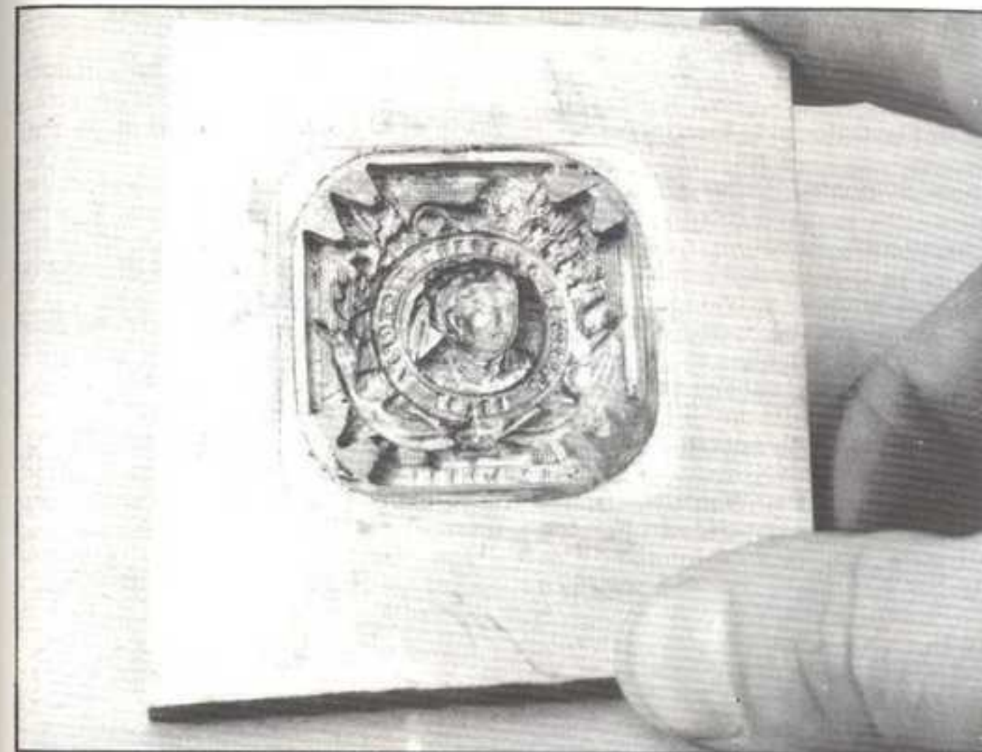
A mould made from a medal by electroforming, set in a backing die allowing it to be used for making a quantity of mouldings in various moulding materials.
