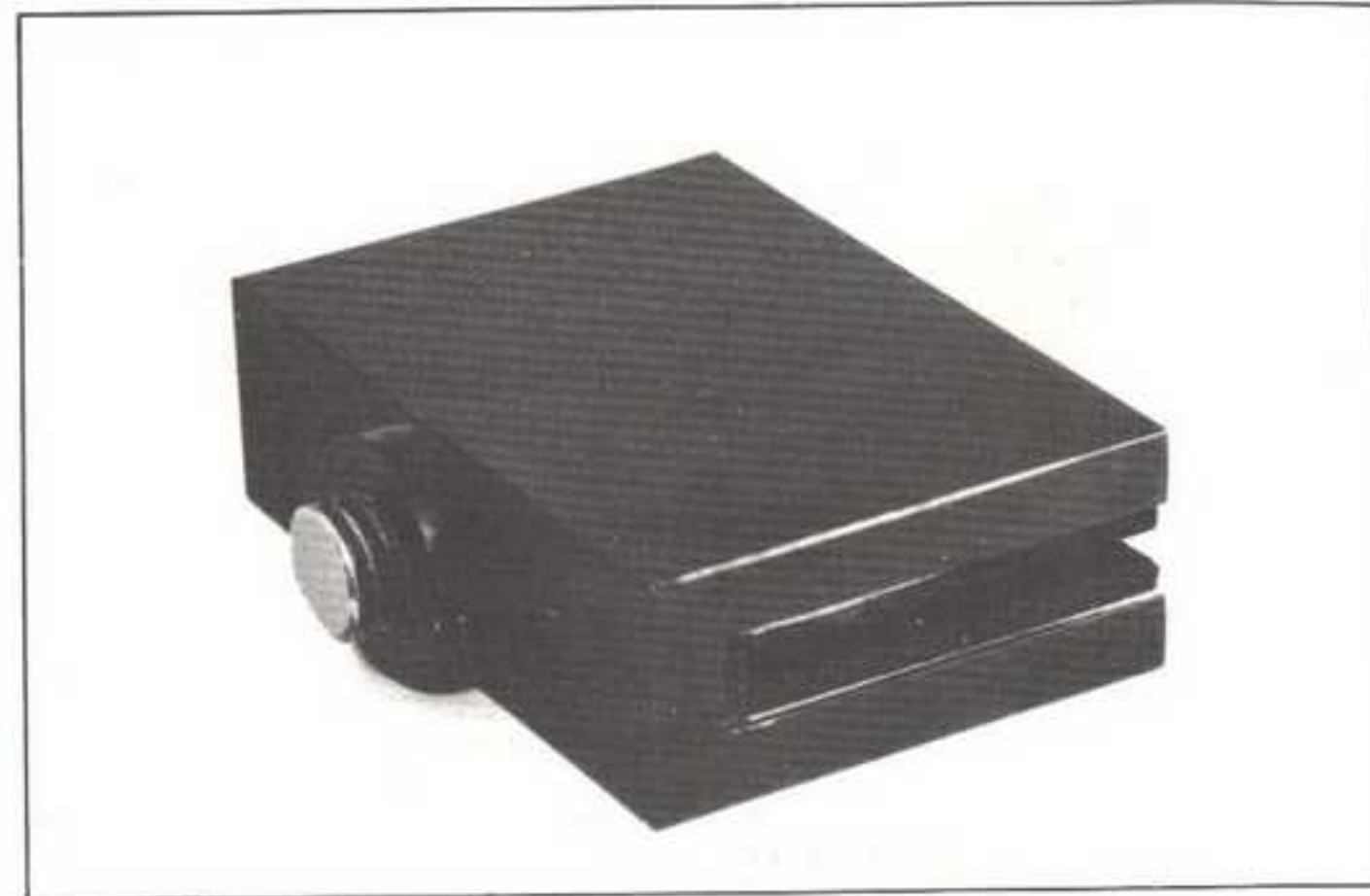
An aluminium component anodised and dyed black following the procedures described.
