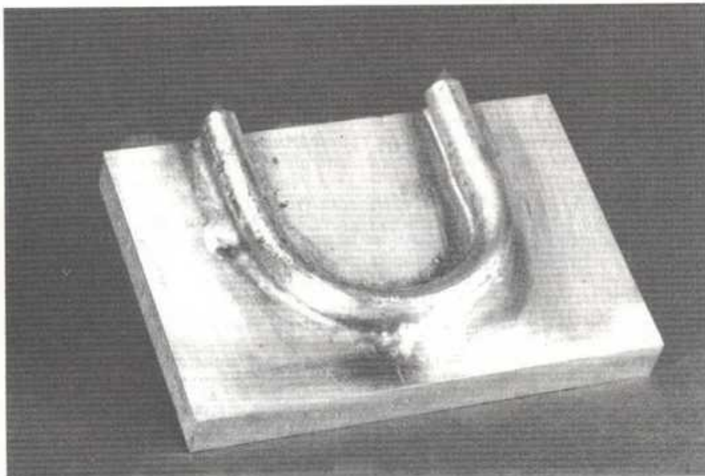
An example of electroplating on aluminium to facilitate soldering. This utilises zincate solution, followed by a layer of tin, with tinned copper tube soldered onto the final tin layer on the aluminium.
