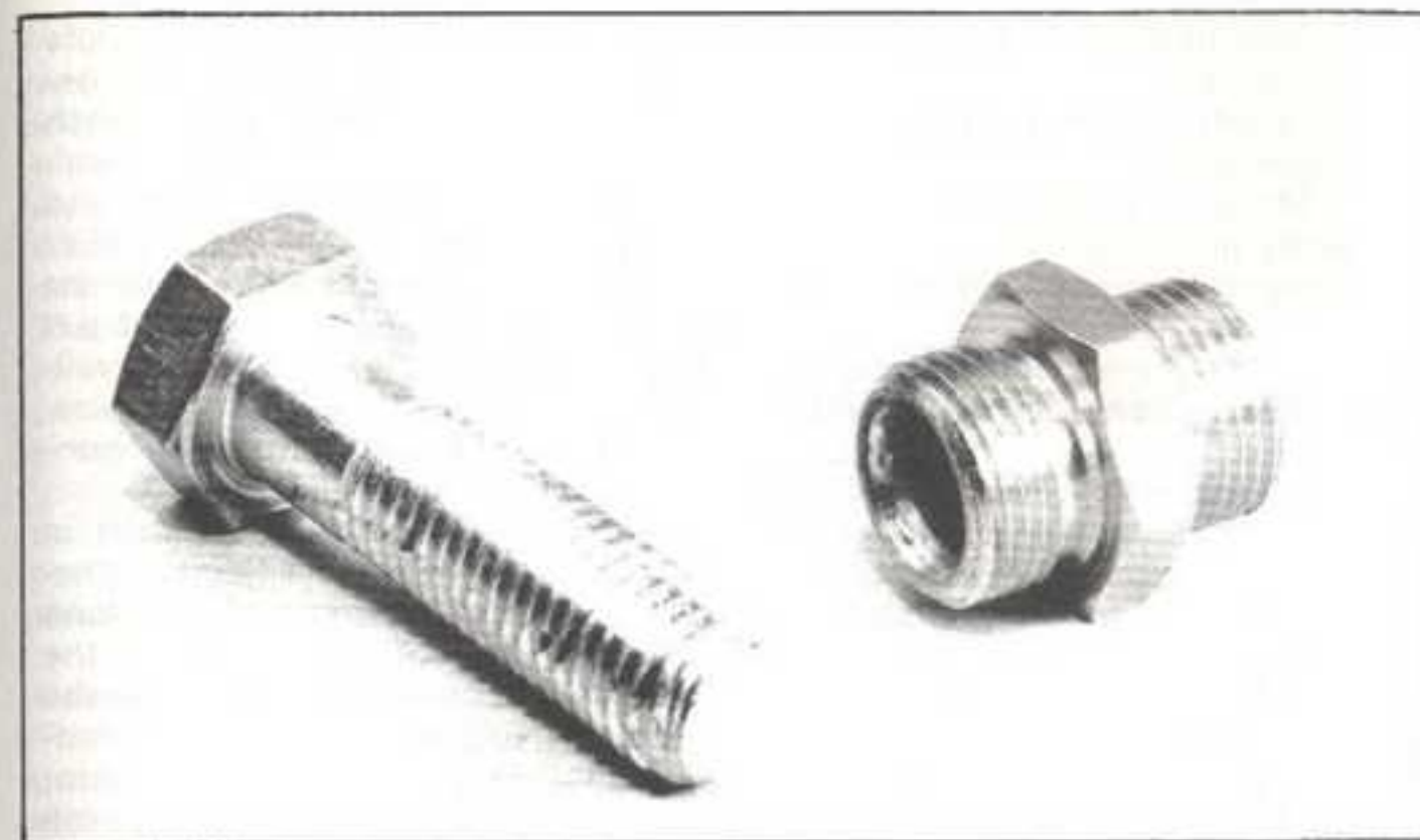
Examples of zinc and passivate and semi-bright nickel. The bolt is electroplated with zinc, and blue passivated. The adaptor is electroplated with semi-bright nickel from the electrolytes described in this chapter.
