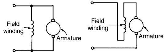
(a) Shunt-wound machine (b) Series-wound machine
