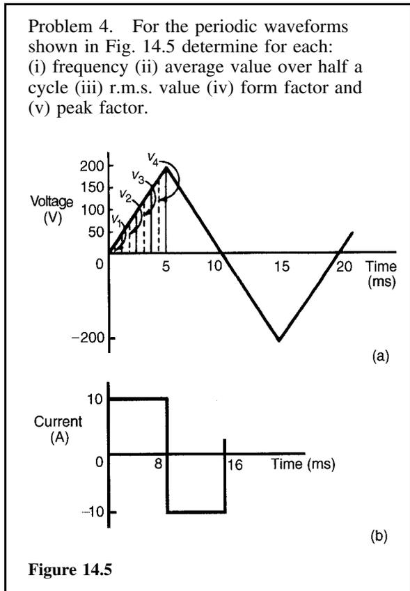
(a) **Triangular waveform** (Fig. 14.5(a)).
