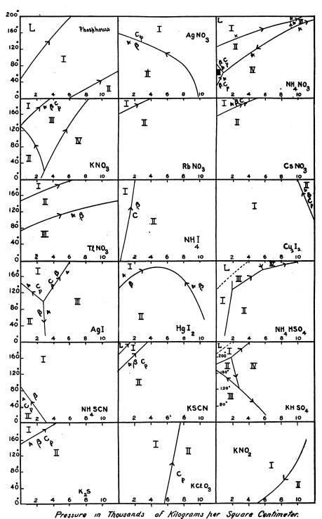
is concave toward the pressure axis, and rises continuously, and the two known falling melting curves are also concave downward. We have here examples of rising and falling curves with curvature in either direction, curves with a maximum temperature (HgI<sub>2</sub>), and curves with a maximum or minimum pressure (H<sub>2</sub>O and Benzol). No cases have
