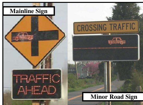
FIGURE 107. Collision Countermeasure System tested in Virginia (79)
