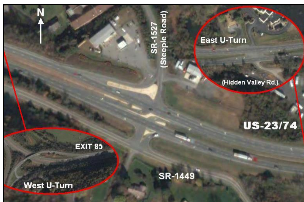
FIGURE 45. Aerial photo of J-turn intersection at US-23/74 & SR-1527/1449
