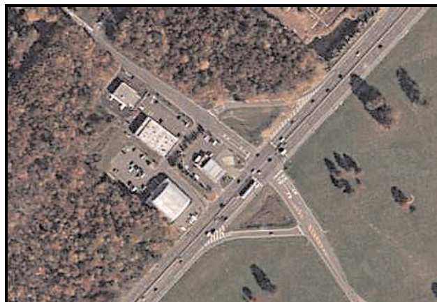
FIGURE 63. Aerial photo of near-side jughandle intersection (30)
