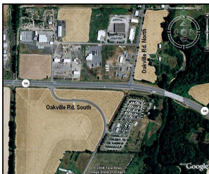
FIGURE 56. Aerial photo of R-L offset T-intersection in Oregon
