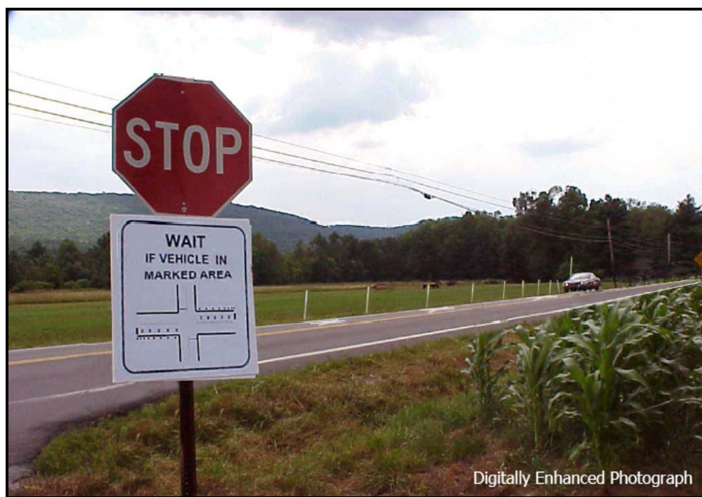
FIGURE 73. PennDOT static gap assistance treatment application (82)
