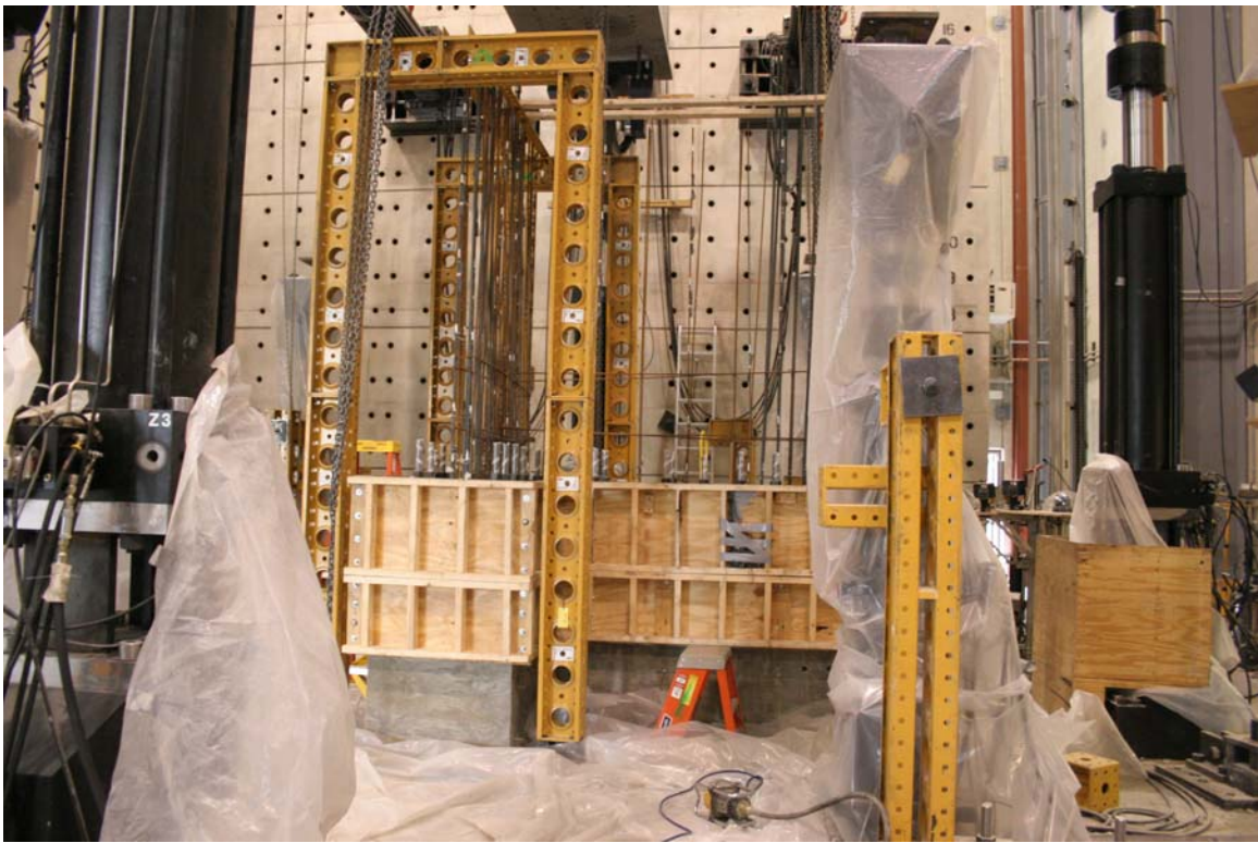
Figure 5-2: Two-part Base Block used for NTW2 to Expedite Construction
