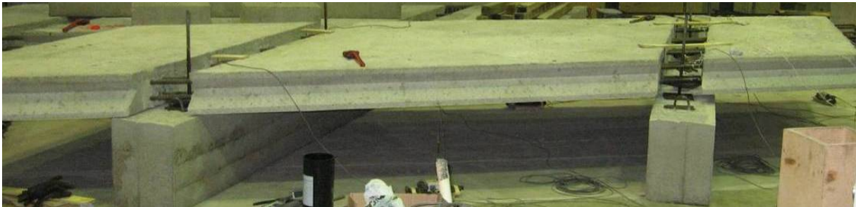
Figure 2.14. Deck panel setup for leveling test.
