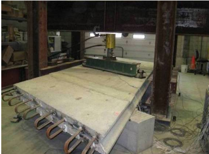
b) Panel 3 setup prior to testing
