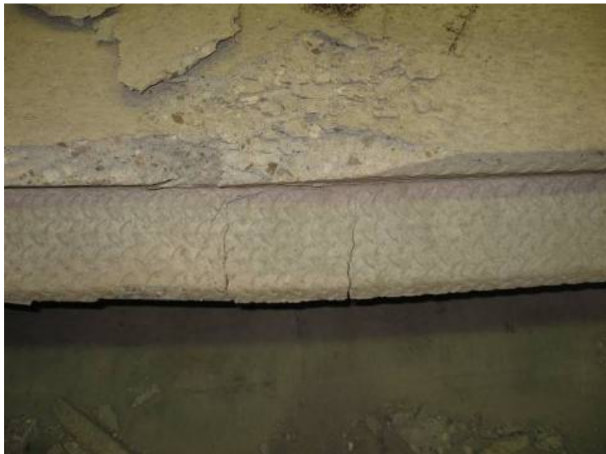
a) deck panel after loading
