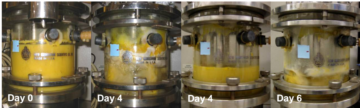
Figure 2. Thin stillage in 1.75-L vessel (1.25-L working volume) started from mycelia on day 0 with biomass removed on day 4. Liquid was returned to the reactor for additional bioconversion of the organic materials to fungal biomass.
