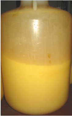
Figure 4.1. Thin stillage suspended solids settled during storage for 1 d in a sterile 20-L carboy at 4°C.
