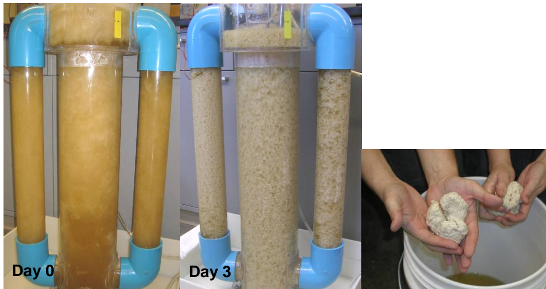
Figure 4.9. Exp. set 2: scaled-up airlift fungal bioreactor cultivating settled thin-stillage supernatant (24 L) with 0.8-vvm aeration on the day of mycelia inoculation (day 0) and filled with mycelia on day 3. The fungal pellets collected on day 3 were separated by coarse screens and dewatered to 20–30% solids by hand squeezing.
