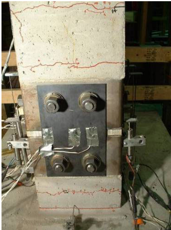
a.) West face cracking at the end of Test 5a
