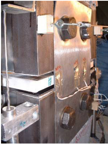
a.) Northeast corner joint opening
