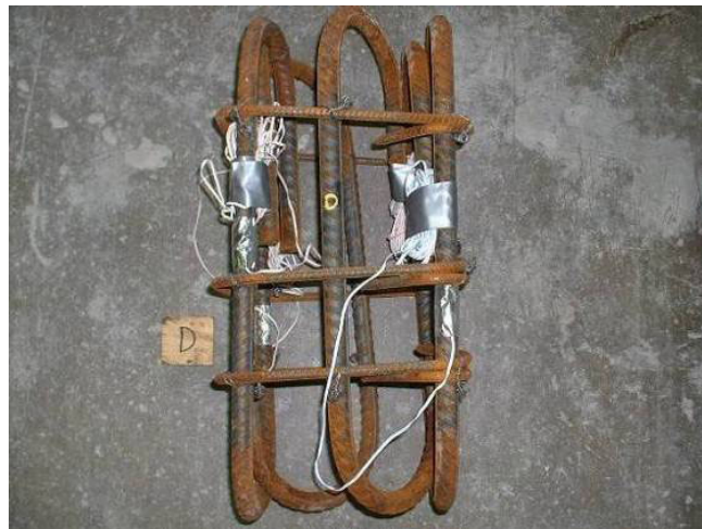
Figure 42. Photograph of Column 3, 2 ft. segment reinforcement.
