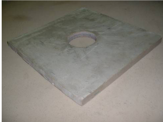
Figure 63. Photograph of epoxy grout plate.
