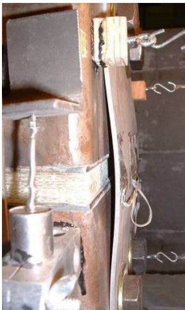
a.) West fuse plate buckling
