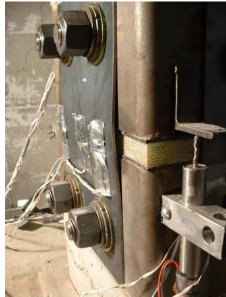
b.) East plate initial buckling
