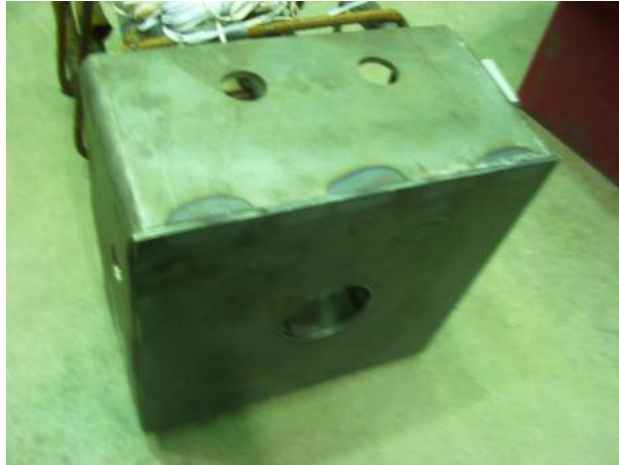
Figure 58 Photograph of Column 6 collar and end plate.
