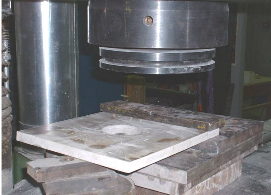
Figure 61. Photograph of edge compression test.
