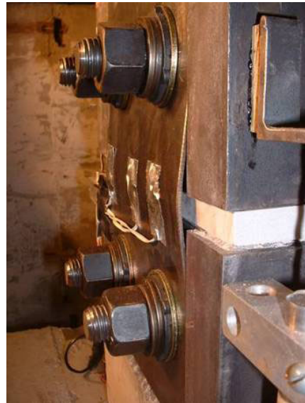
b.) Initial buckling of east plate
