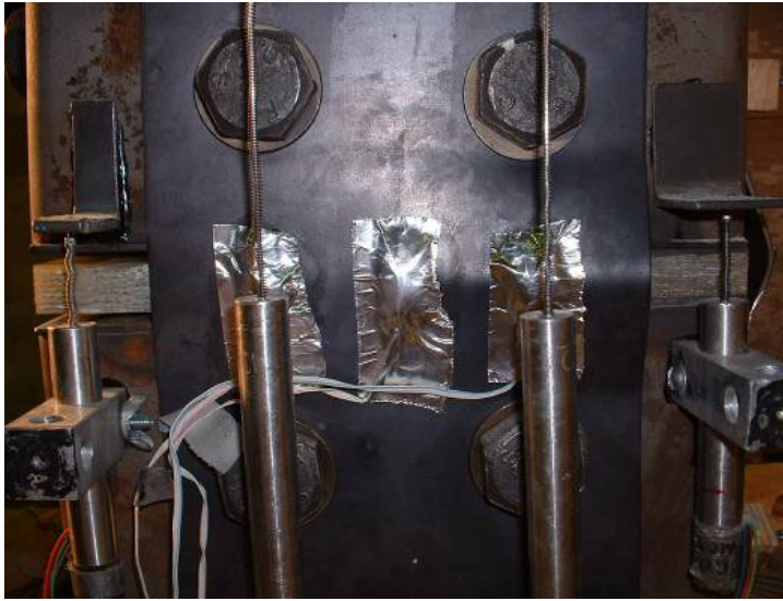
a.) Differential buckling in north fuse plate buckling
