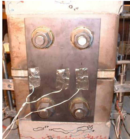
b.) East joint opening during push half-cycle
