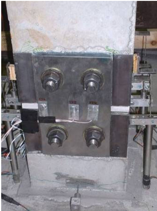
a.) East replacement fuse plate
