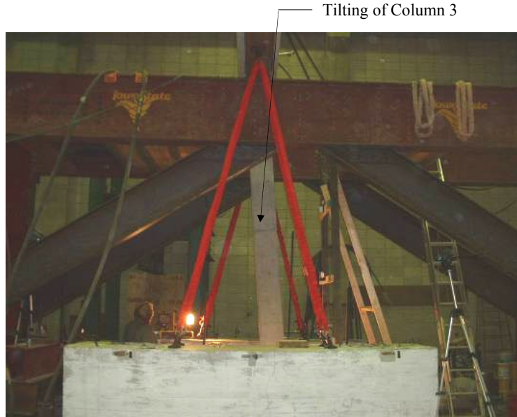
b.) Pull half-cycle column deformation
