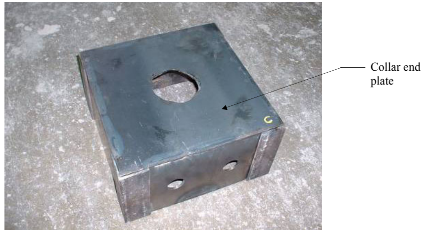
Figure 41. Photograph of Column 3 collar and end plate.
