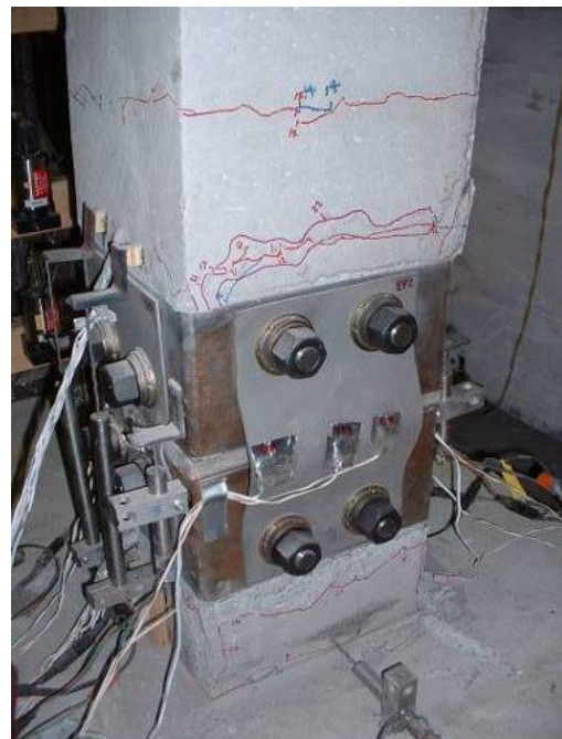
b.) East face under compression
