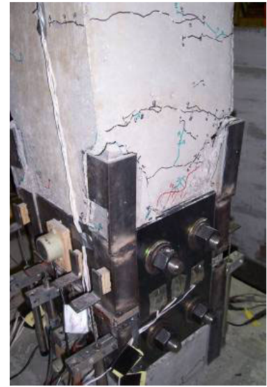
b.) East face column damage
