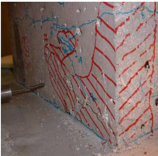
a.) Southwest corner compression damage
