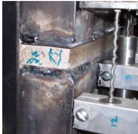
b.) Northeast corner bearing plate compression damage
