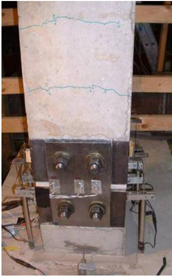
a.) East face crack progression
