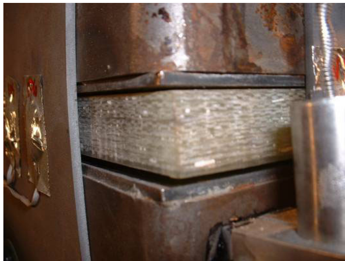
Figure 150. Photographs of Column 6 – Cycle 21b, joint opening.
