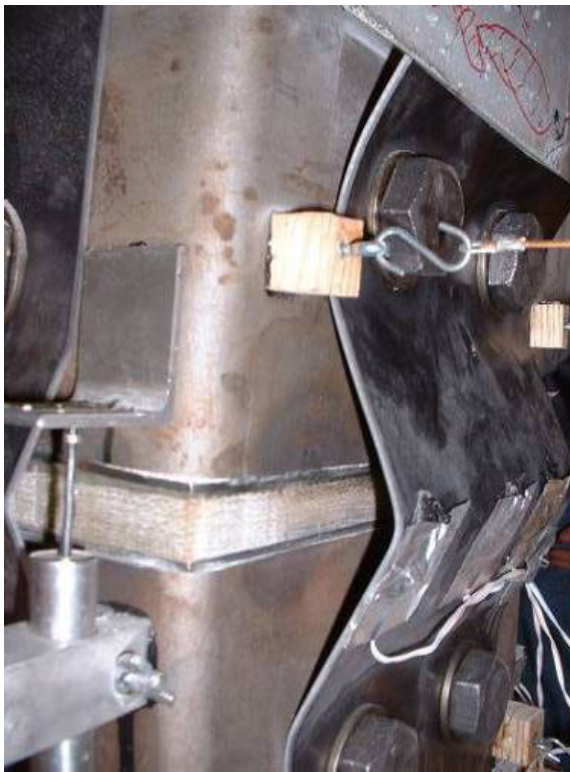
b.) West fuse plate buckling during push half-cycle
