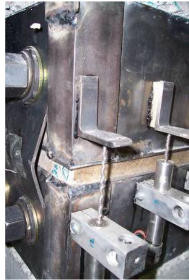
d.) Northeast corner fuse plate buckling
