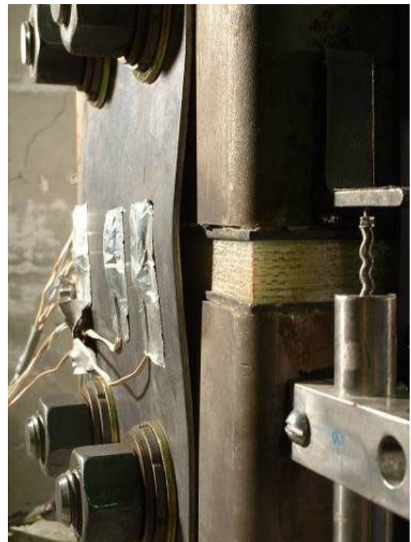
b.) East plate buckling in compression
