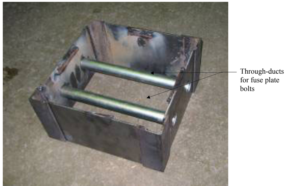
Figure 40. Photograph of Column 2 steel collar with bolt through-ducts.
