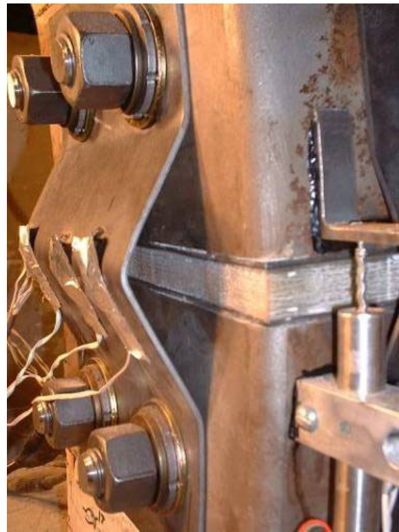
c.) East fuse plate buckling during pull half-cycle
