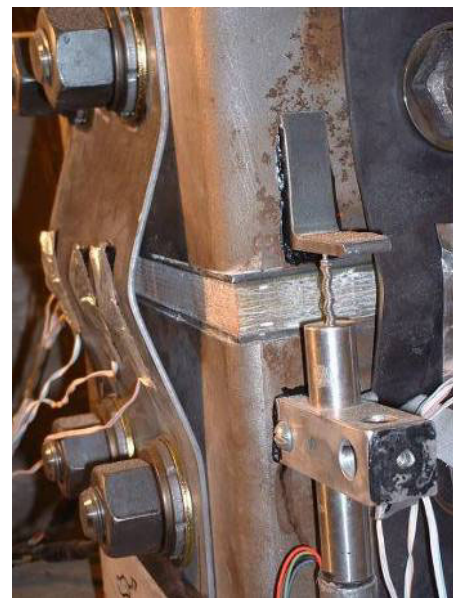
d.) Northeast corner fuse plate buckling
