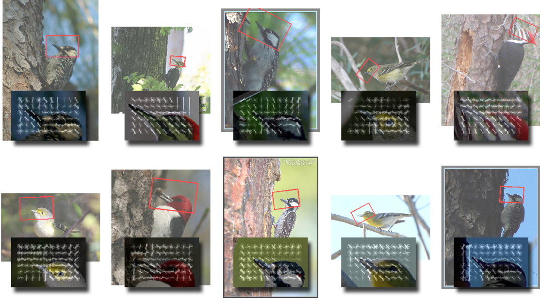
Figure 2.4: Birdlet Training . This illustration shows the process of selecting the positive training set. Training examples with similar pose (within the window of interest) are identified and an aligning similarity transform determined. Then for each training example, a HOG description is extracted for the aligned patch. These features collectively form the positive training set.
