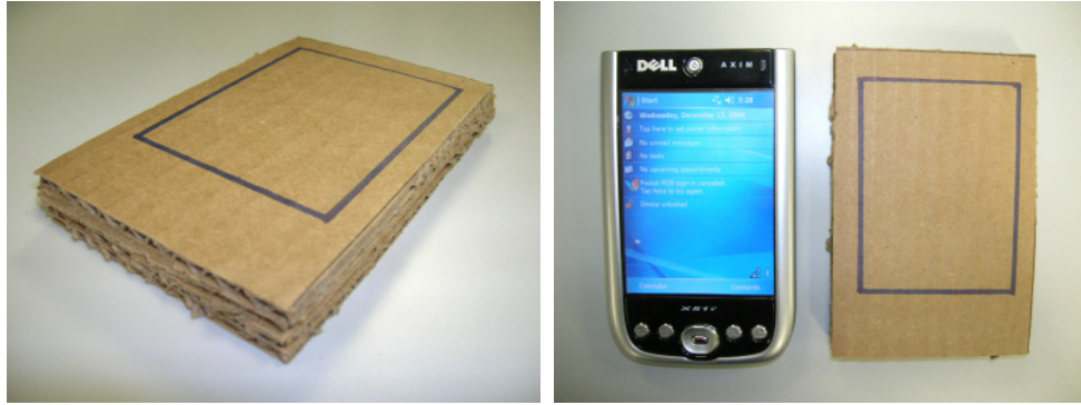
Figure 3.20 – Low-fidelity version of mobile device, used in low-tech and paper prototyping sessions
