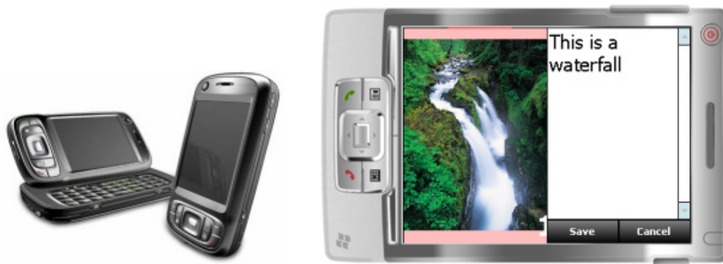
Figure 3.30 – Landscape layout while editing text: left , fold out keyboard; right , editing text when keyboard is extended.
