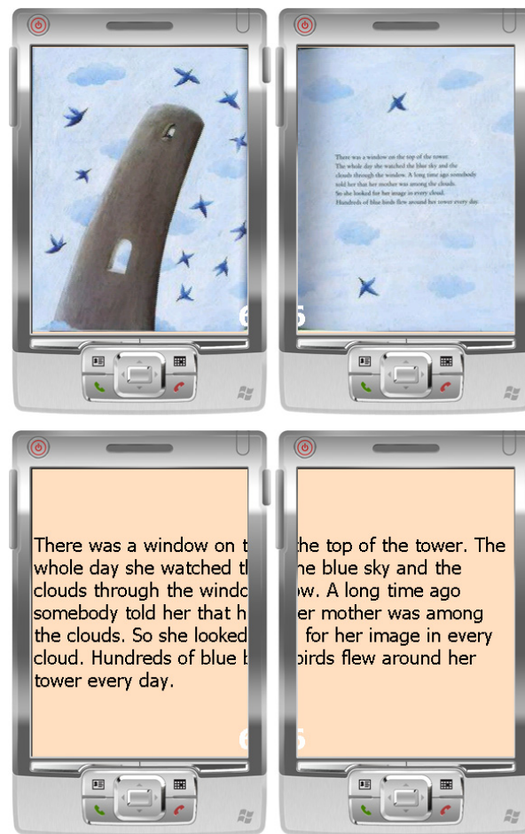
Figure 1.3 – Space Sharing, mobile collaboration using a page from the same book as in Figure 1.2; top , an image; bottom , words spread across both devices.
