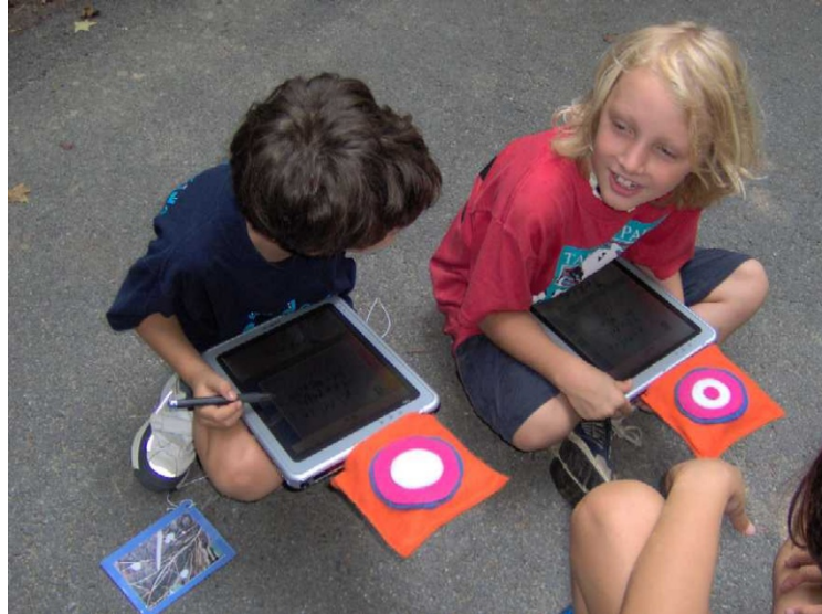
Figure 3.6 – Children using Tangible Flags, the bulls-eye is an RFID reader, the blue flag has an RFID card inside; the children are both adding annotations to the same flag.
