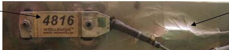
(b) BDI strain transducer installed next to the weldable strain gage
