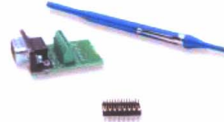
CN-189 and CN-115 header connectors provide bridge completion
