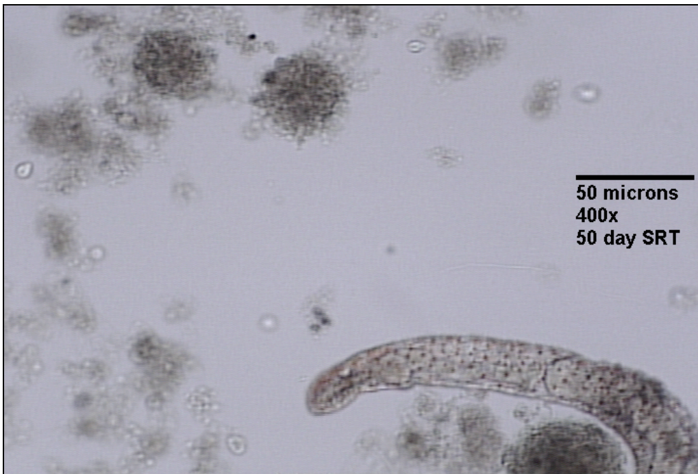
Figure 4.8 Example of microscope image of sludge sample, 50 day SRT
