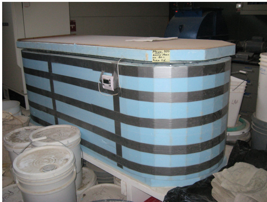
Curing tank for ASR conditioning (50°C and >95% relative humidity)
