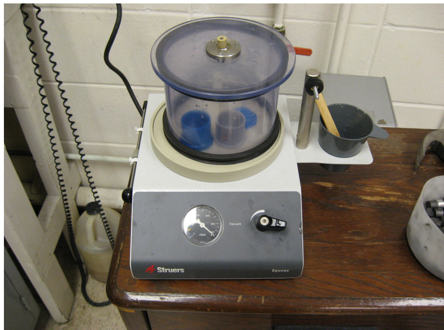
Unit for epoxy impregnation under vacuum
