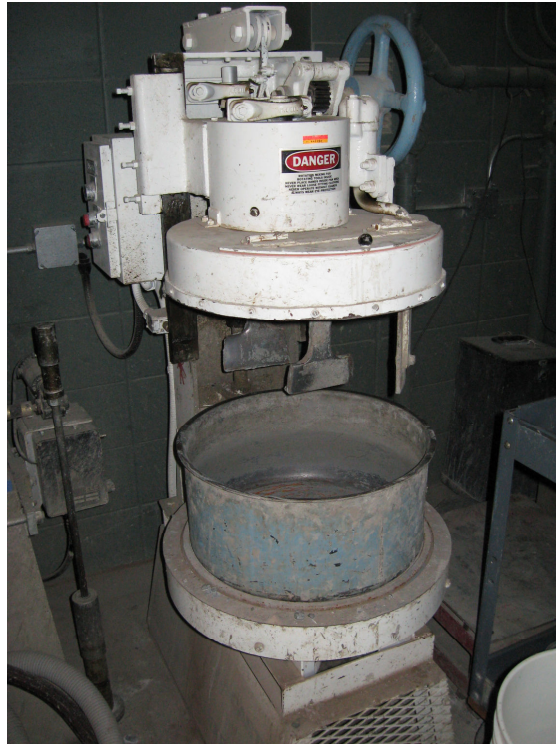
Concrete mixer – pan type
