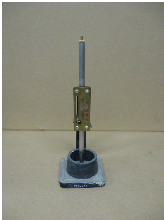
Vicat apparatus for normal consistency and time of setting of cementitious pastes
