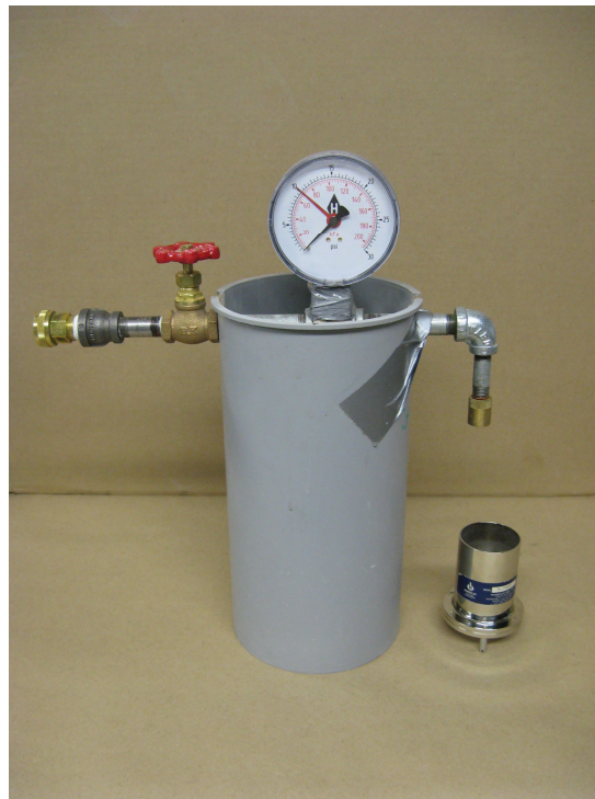
Water pressure regulator and ASTM No. 325 sieve for 45 \mu\text{m} residue analysis
