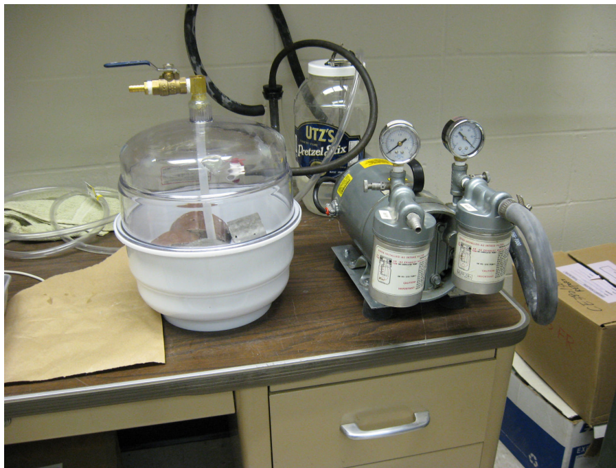
Vacuum pump and desiccator for rapid chloride permeability testing
