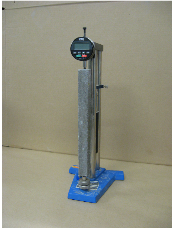
Comparator for length change measurement of mortar-bars and concrete prisms
