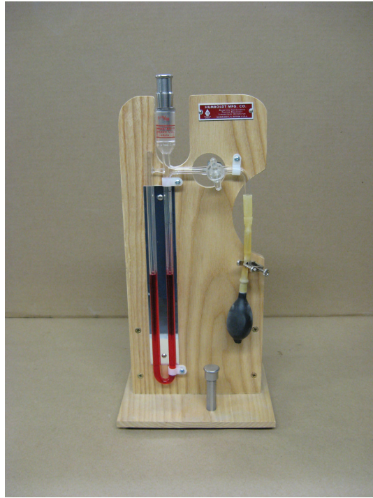
Blaine apparatus used to measure the fineness of portland cement
