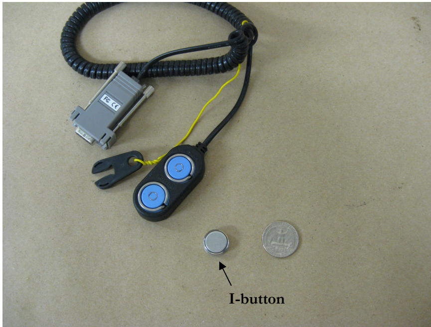
I-button and data collector for temperature measurement during paste hydration
