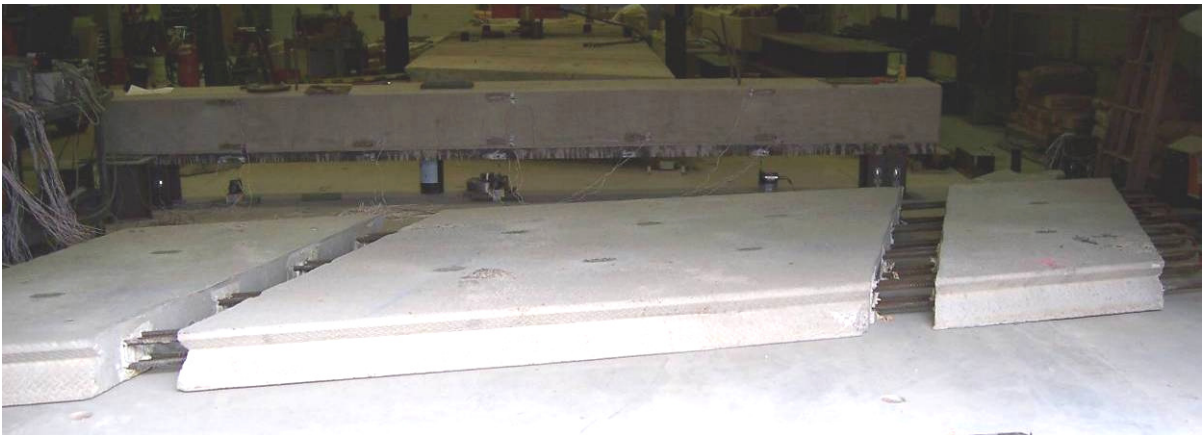
Figure 6. Boone County replacement bridge deck panel.
