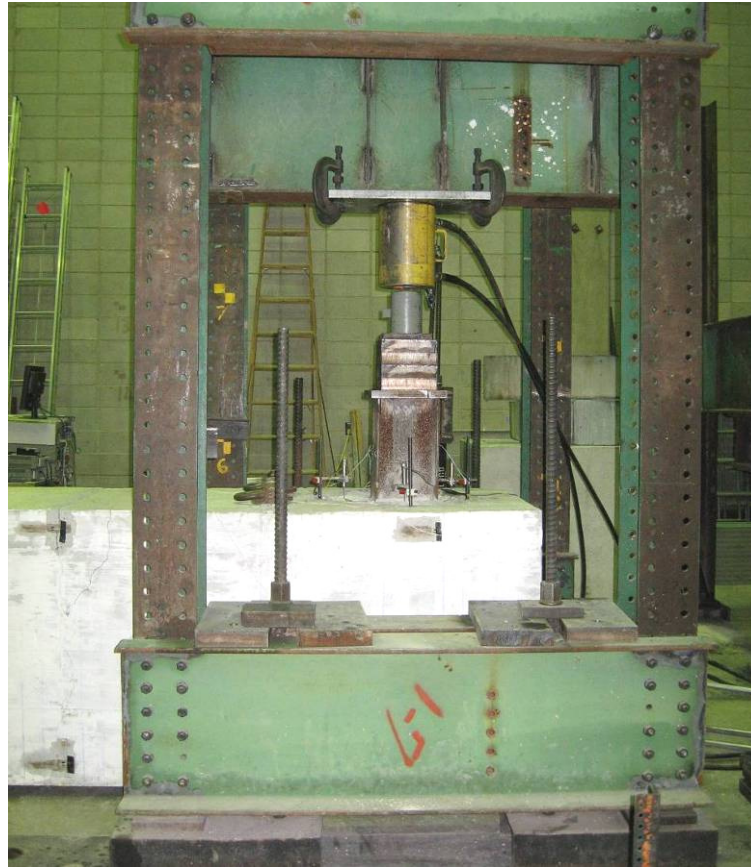
Figure 43. Double pile abutment shear Test 1.
