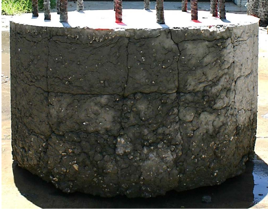
Figure A.18. Shaft 5, 90 sec/qt mineral slurry after pressure washing.
