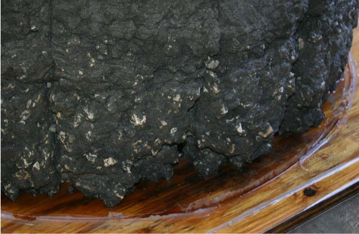
Figure 4.9. 90-second shaft after pressure washing.
