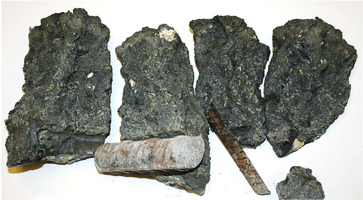
Figure A.32. Core from shaft 9, 50 sec/qt mineral slurry.
