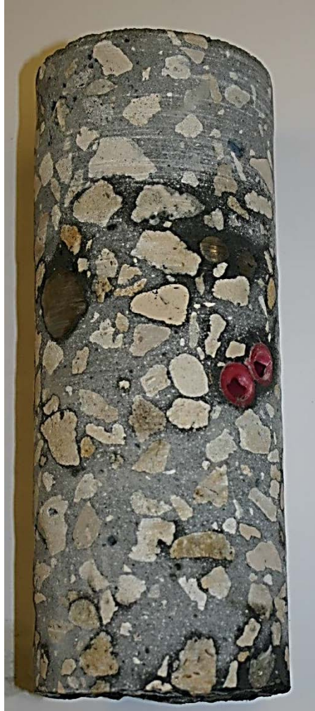
Figure A.29. Core from shaft 11, 60 sec/qt polymer.
