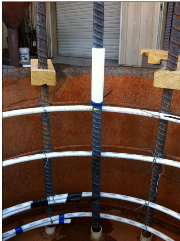
Figure A.7. Typical de-bonding for reinforcement.
