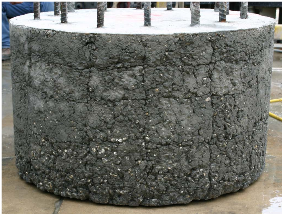
Figure A.21. Shaft 9, 50 sec/qt mineral slurry after pressure washing.
