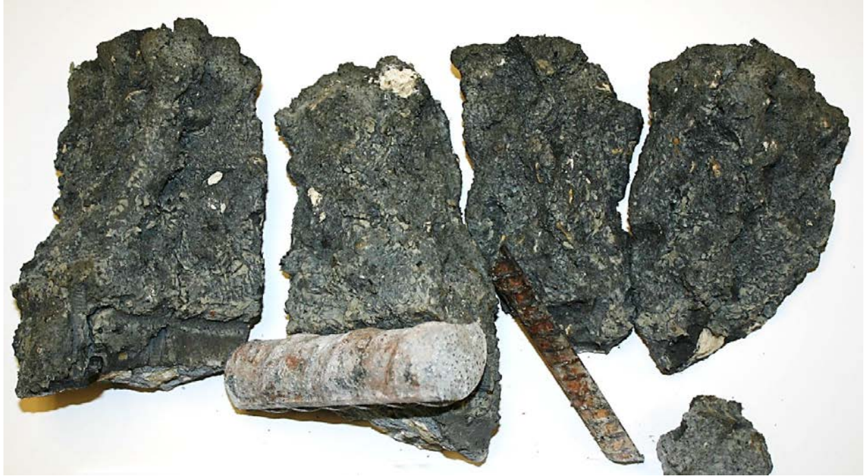
Figure 5.11. Encapsulated slurry in 50 sec/qt shaft core.
