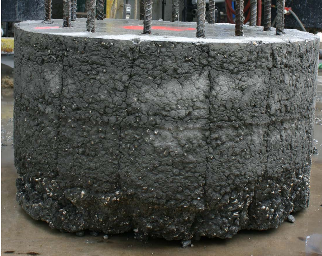
Figure A.22. Shaft 10, 90 sec/qt mineral slurry after pressure washing.
