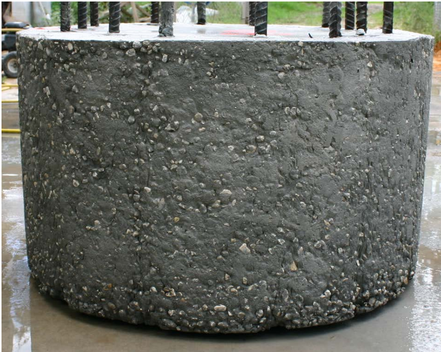
Figure A.19. Shaft 7, 30 sec/qt mineral slurry after pressure washing.
