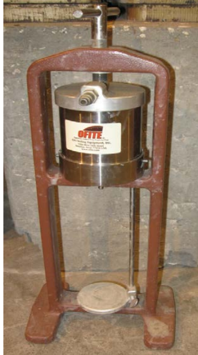
Figure 2.7. Bench top filter press.
