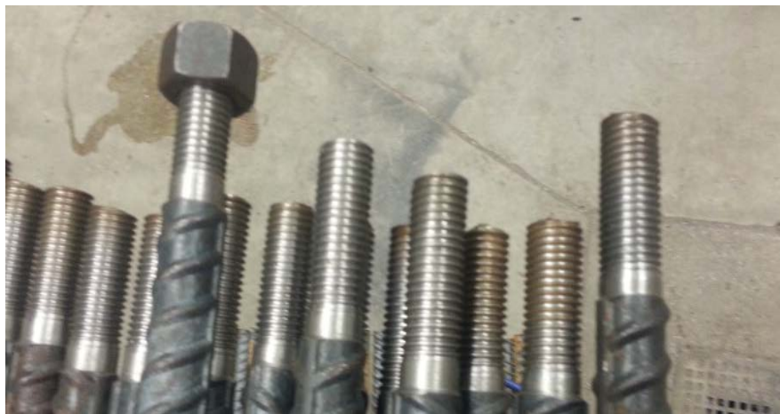
Figure 3.7. Reinforcement after machining.
