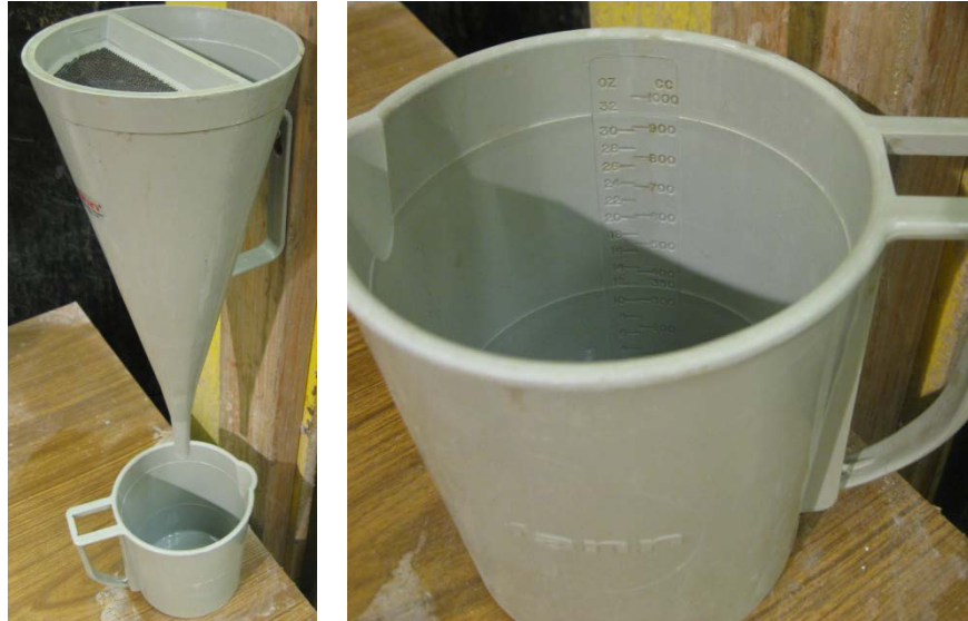
Figure 2.3. Marsh funnel and cup for determining viscosity.
