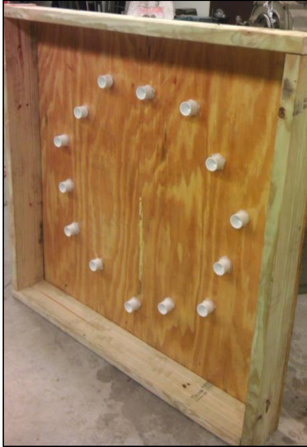
Figure A.4. Bottom of form after polyurethane and cap placement.
