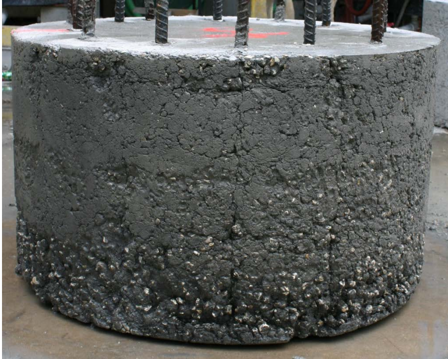
Figure A.20. Shaft 8, 40 sec/qt mineral slurry after pressure washing.
