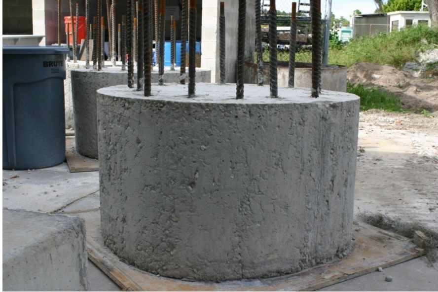
Figure A.24. Shaft 13, 30 sec/qt mineral slurry after pressure washing.
