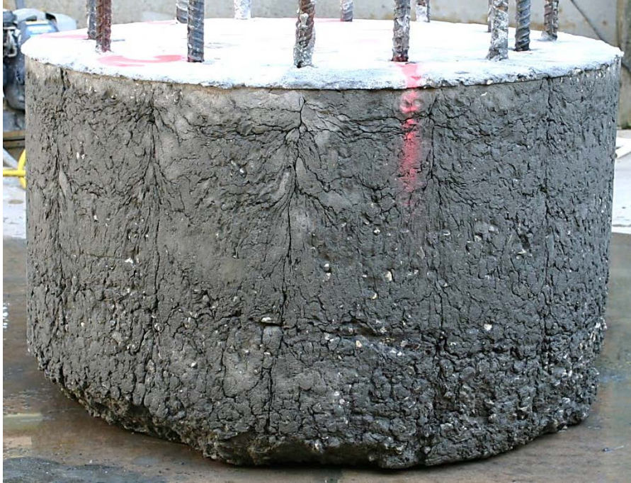
Figure A.16. Shaft 3, 40 sec/qt mineral slurry after pressure washing.
