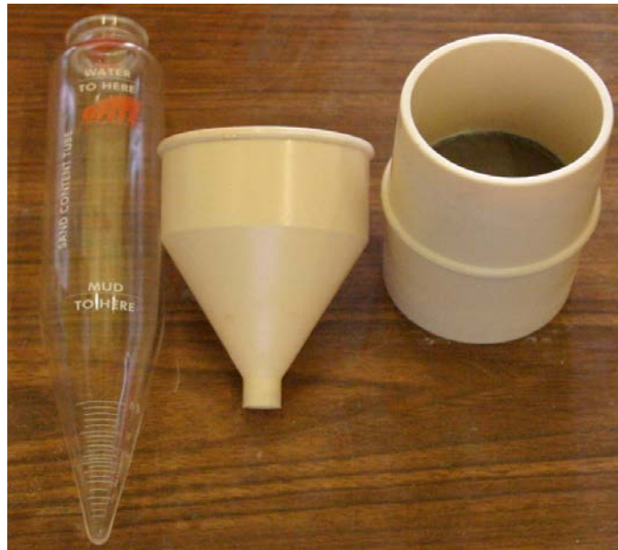
Figure 2.5. Test kit for sand content.
