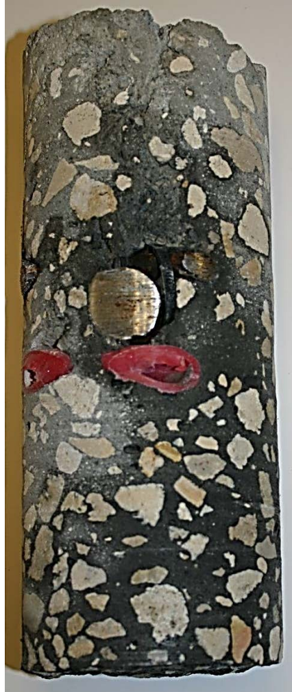
Figure A.31. Core from shaft 8, 40 sec/qt mineral slurry.
