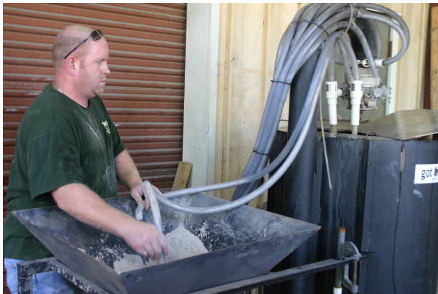
Figure 3.8. Mixing mineral slurry with Hootonanny® eductor.
