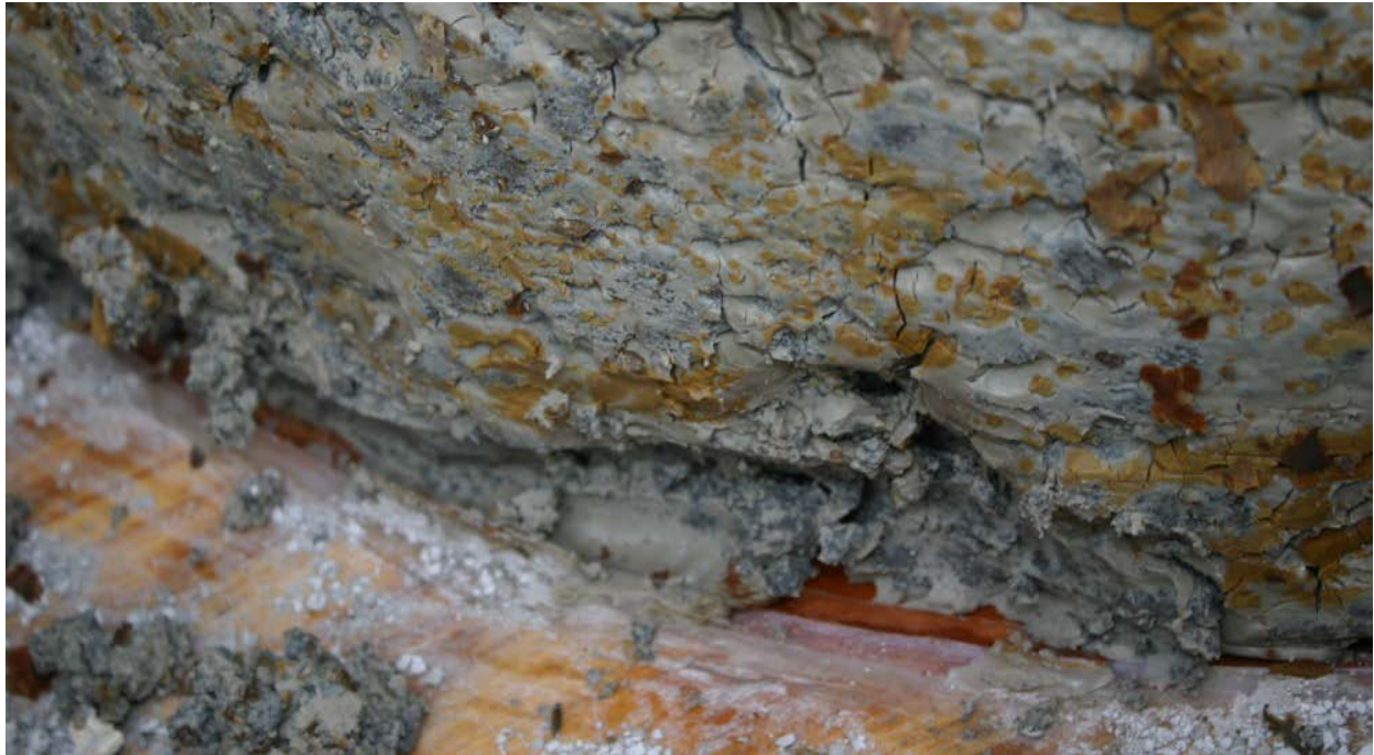
Figure 4.8. Buildup encountered at bottom of 90-second shaft from placement one.
