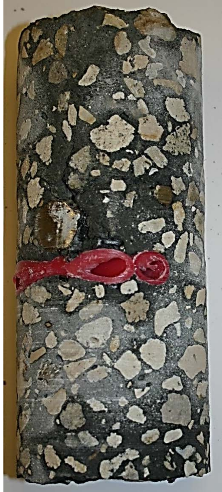
Figure A.30. Core from shaft 7, 30 sec/qt mineral slurry.
