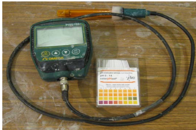
Figure 2.6. pH meter (left) and litmus strips (right).
