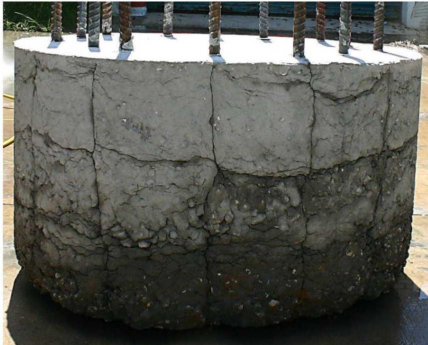
Figure A.17. Shaft 4, 50 sec/qt mineral slurry after pressure washing.
