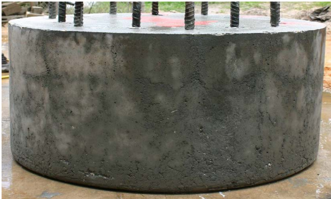
Figure 5.8. Illustrates the consolidation of the 60 sec/qt polymer shaft.
