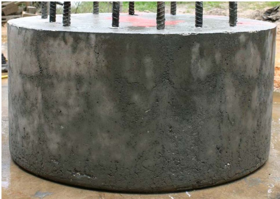
Figure A.23. Shaft 11, 60 sec/qt polymer slurry after pressure washing.
