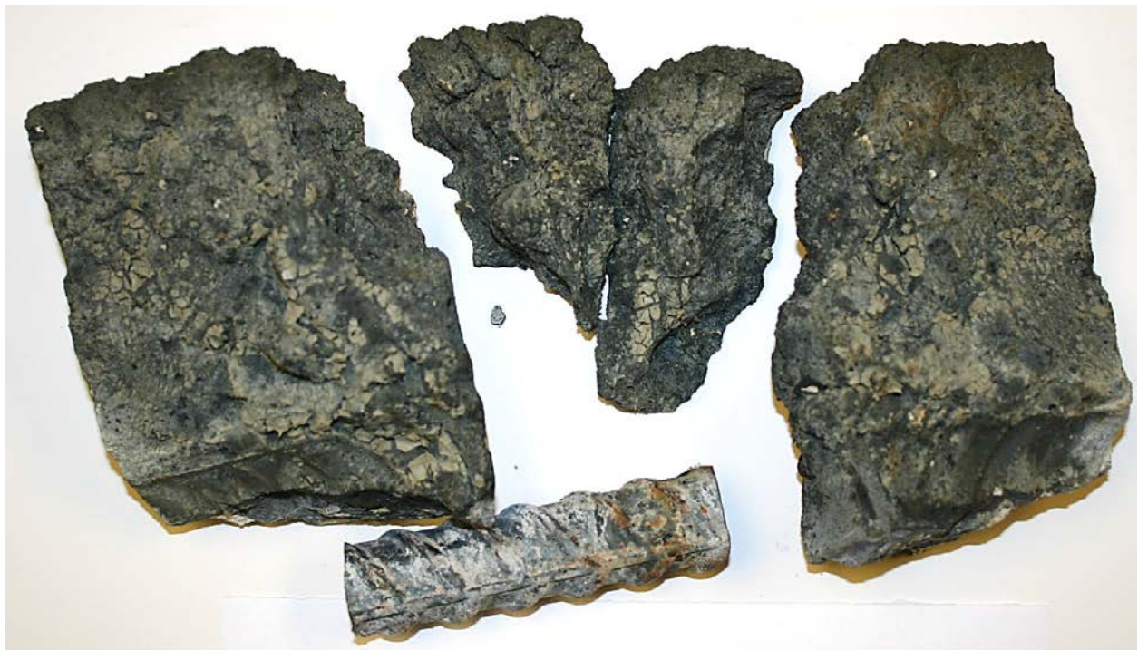
Figure A.33. Core from shaft 10, 90 sec/qt mineral slurry.
