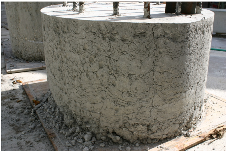
Figure A.25. Shaft 15, 50 sec/qt mineral slurry after pressure washing.
