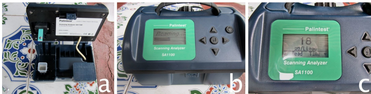
Figure 15. ASV process: a) the ASV unit with electrode in place and sample prepared; b) sample processing; c) corresponding measurement of dissolved Pb concentration.
