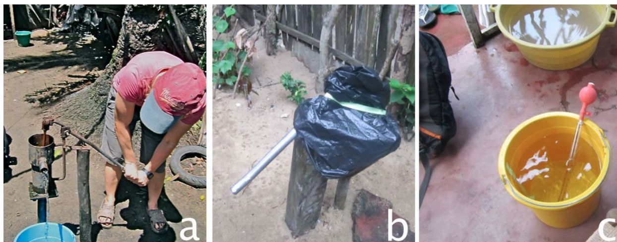
Figure 9. Sample collection and preparation: a) flushing of the pump by Meghan Wahlstrom-Ramler; b) “closed” pump during the 1-hour waiting period after flushed sample collection; c) preparation of a drawn sample with a pipette.
