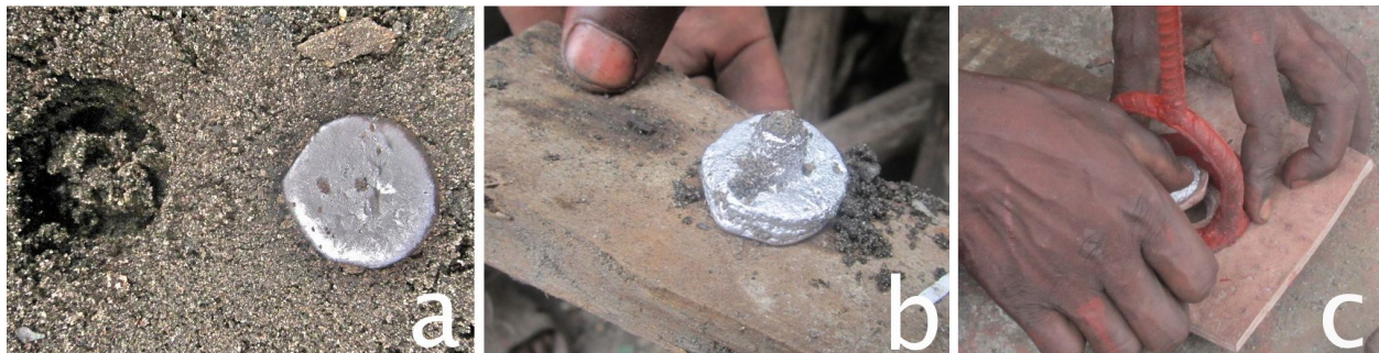
Figure 12. Typical fabrication of Pb valve weights: a) sand-casting of molten Pb; b) removal of sand-casted Pb valve weight seconds after pouring; c) installation of Pb into piston valve.
