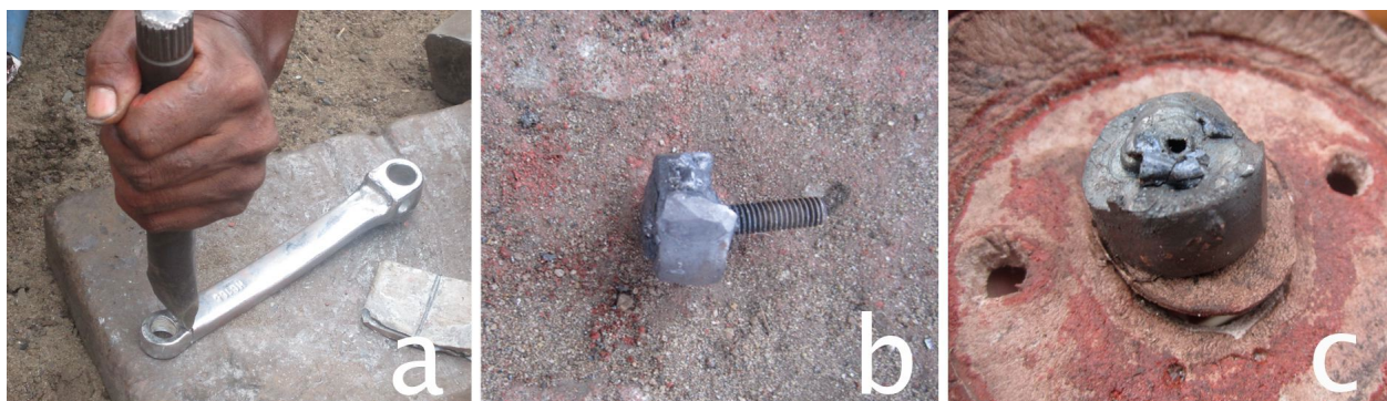
Figure 13. Fabrication of Fe valve weights: a) use of an old galvanized wrench; b) use of nut and bolt; c) representation of a finished foot valve with Fe weight.
