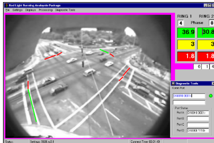
Figure 18. RLRAP monitoring an intersection (58).
