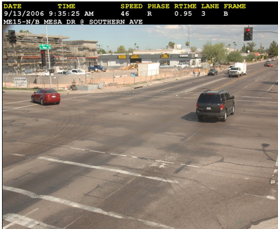
Figure 13. Second picture taken by an automated RLR enforcement camera (Mesa, AZ).
