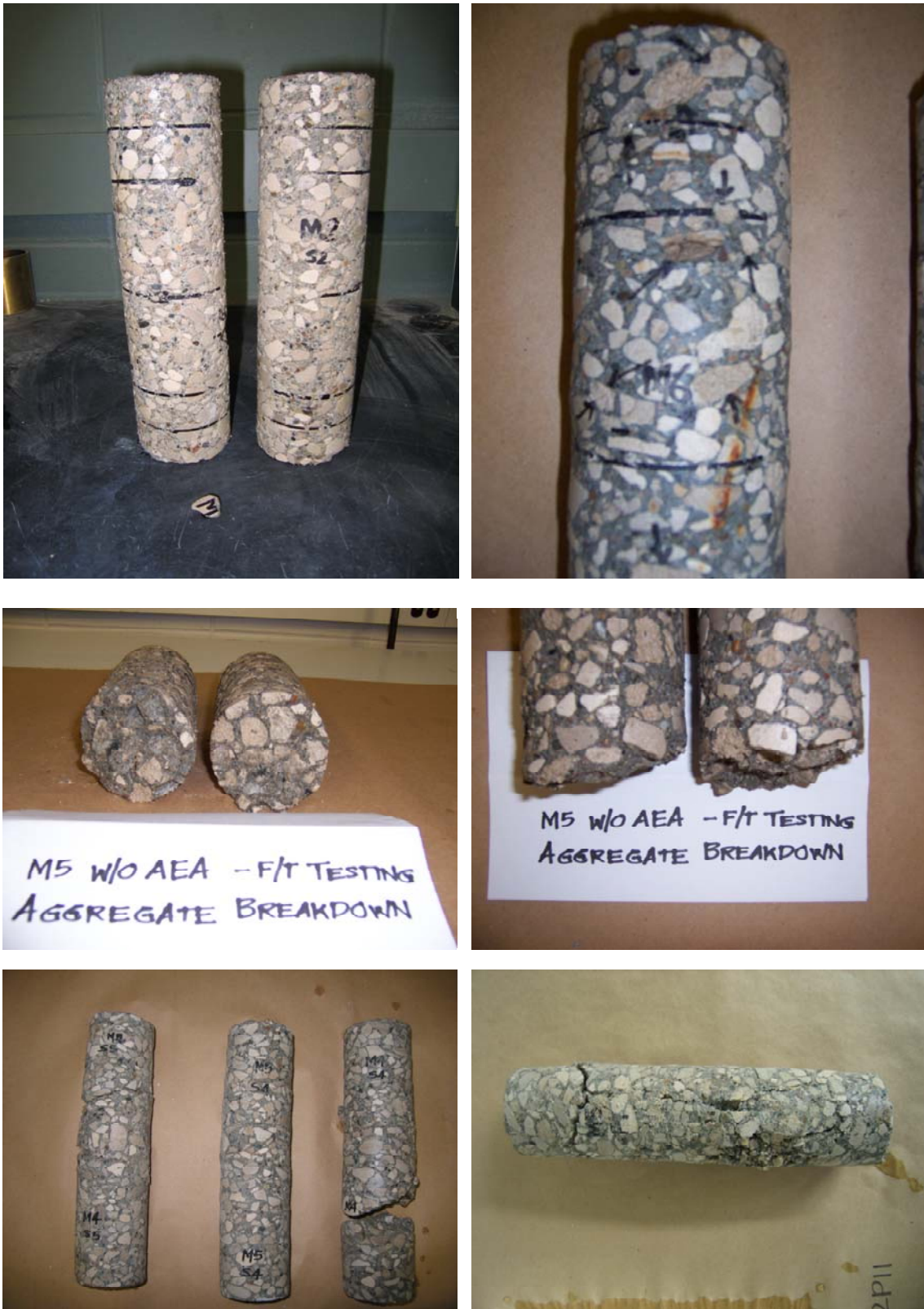
Figure 60 Modes of failures due to F-T loading
