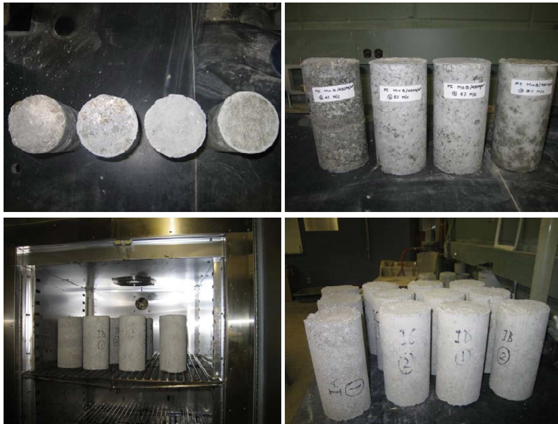
Figure 26 Oven drying of cylinders for moisture content determination
