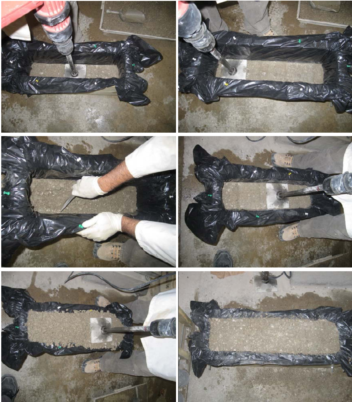
Figure 27 Casting sequence of beam specimens for F-T samples
