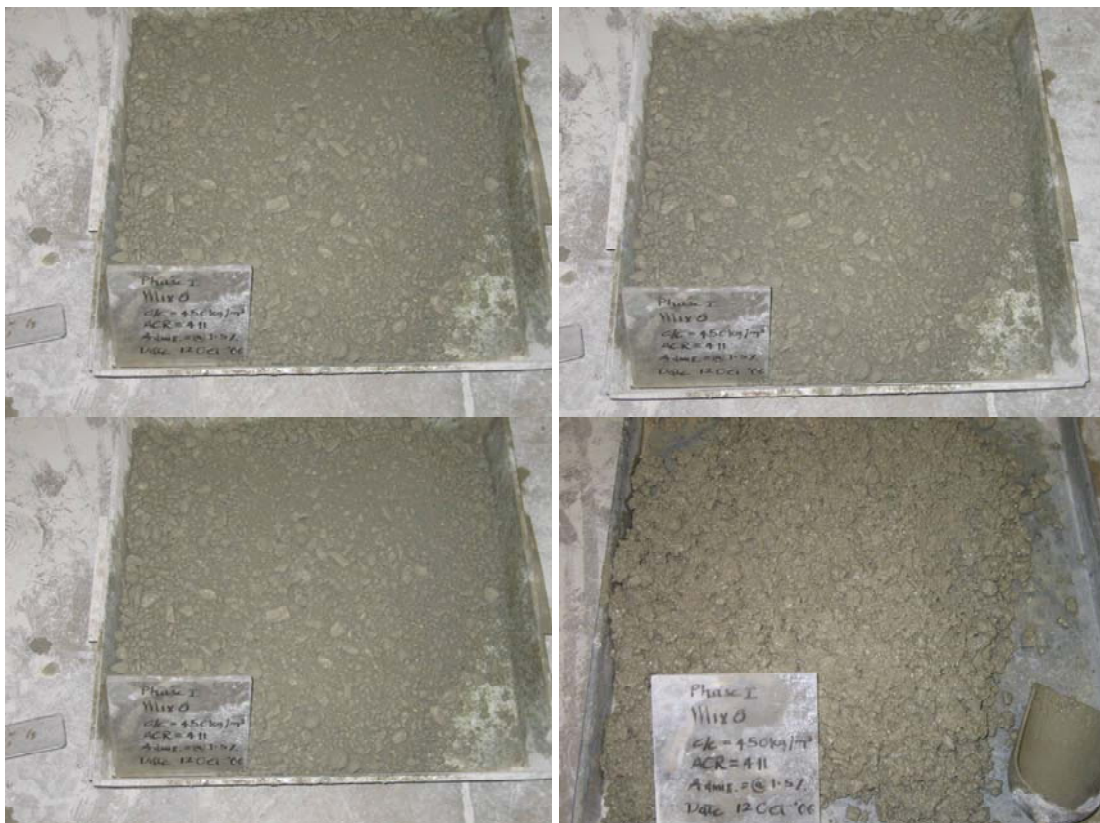
Figure 25 Mixes at different moisture contents
