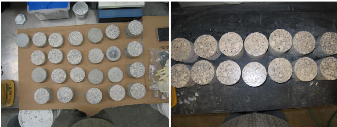
Figure 29 Sample coating for sorptivity samples
