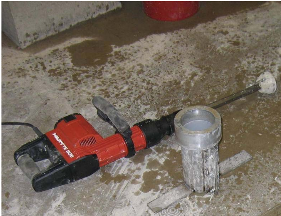
Figure 24 Compacting hammer, steel sleeve and a cylinder
