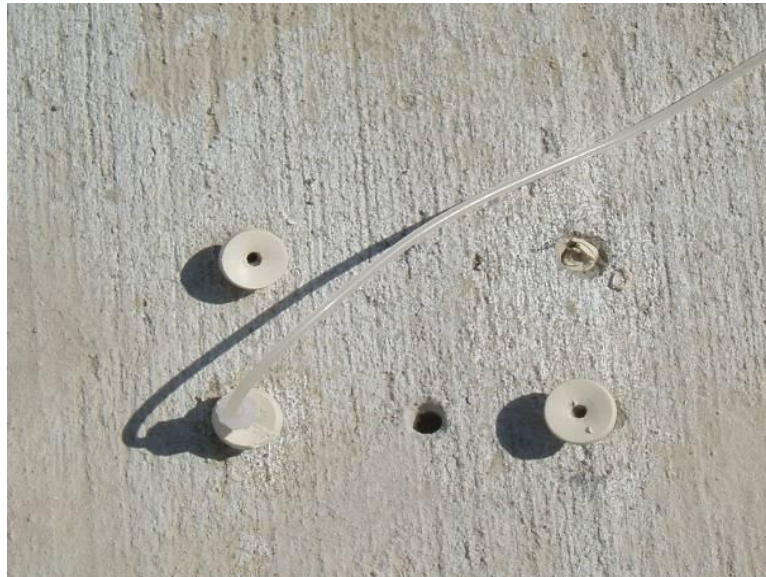
Figure 4.8 Permeability Meter Plug Configuration
