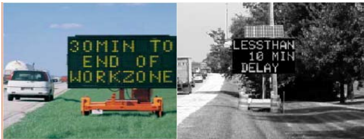
Figure 7. Travel Time and Delay Estimation Displays (52)
