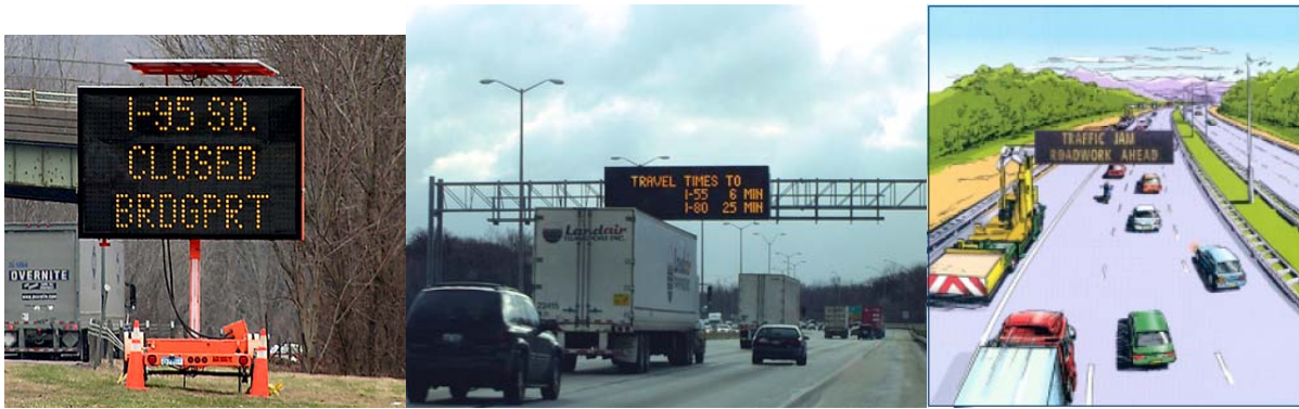
Figure 5. Dynamic Message Signs: Portable, Fixed Overhead (50) and Portable Sign Gantry (49)
