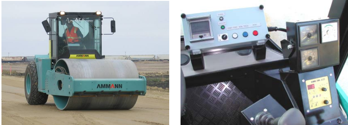
Figure 2.1. Ammann vibratory smooth drum roller with integrated ACE system
