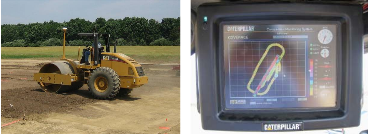
Figure 5.1. Caterpillar CS-533 vibratory smooth drum roller with compaction monitoring technology
