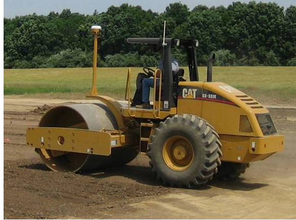
Figure 6.5. Caterpillar CS-533 vibratory smooth drum roller
