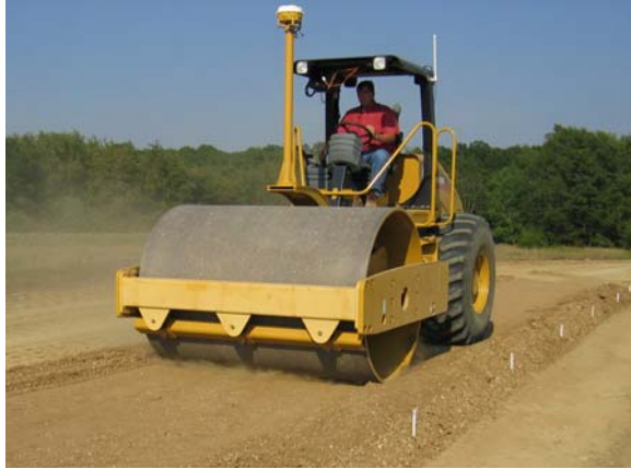
Figure 3.1. Prototype CS-533E vibratory smooth drum roller with roller integrated compaction monitoring technology
