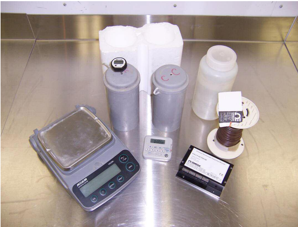
Figure 3-2. Laboratory Test Equipment used to Conduct the Quick Heat Generation Test
