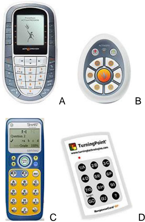
Figure 2-1. Examples of learner response systems. A) Promethean's ActivExpression® and B) ActiVote®, C) SMART's Senteo® and D) Turning Point Response Pad.
