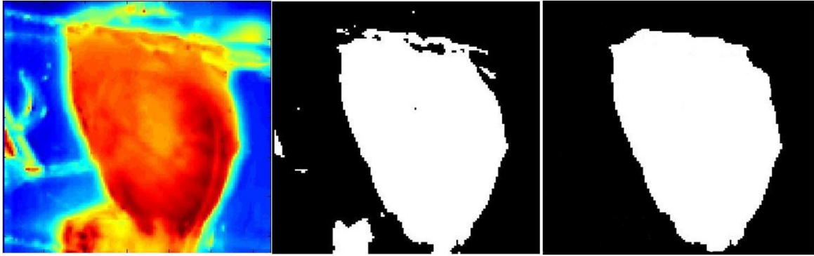
Figure 7 Example of mask generation. The process involved importing first 3000 frames of images, followed by computation of cumulative peak-to-peak difference for each pixel in all frames. Results of this operation are plotted in the left panel. The red area is approximately the position of the heart. After this step, an appropriate threshold was selected so that image on the left is converted to a binary image (middle). After applying image morphology operation to the binary image, the tiny holes were filled and noise reduced.
