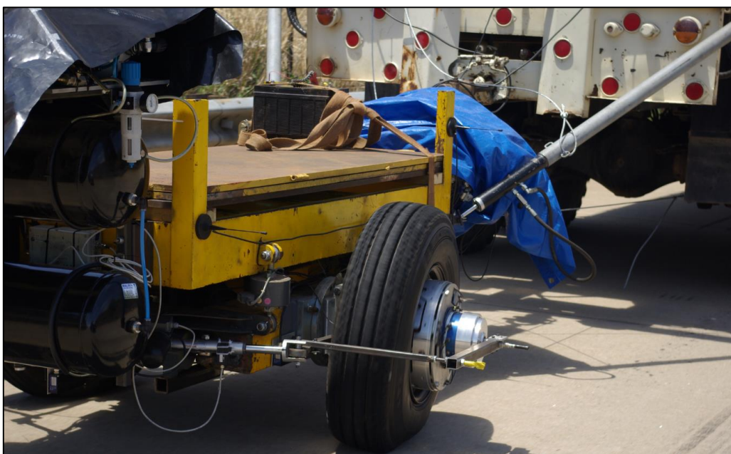
Figure 3-24: Handling validation test (LC3) at 2 bar inflation pressure
