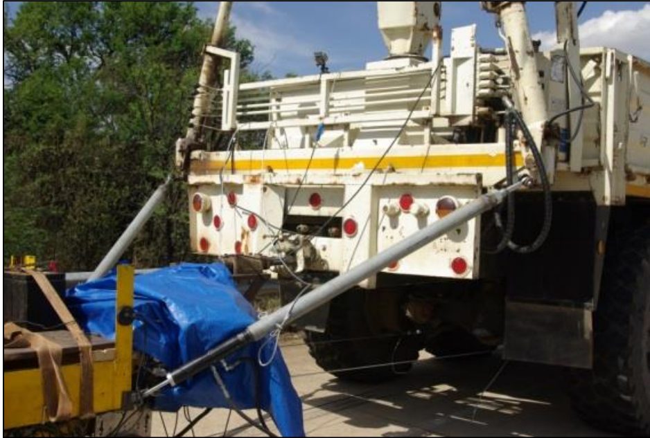
Figure 3-19: Outdoor tyre testing equipment stabilisation system
