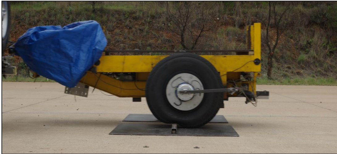
Figure 3-21: Dynamic cleat test (LC0)
