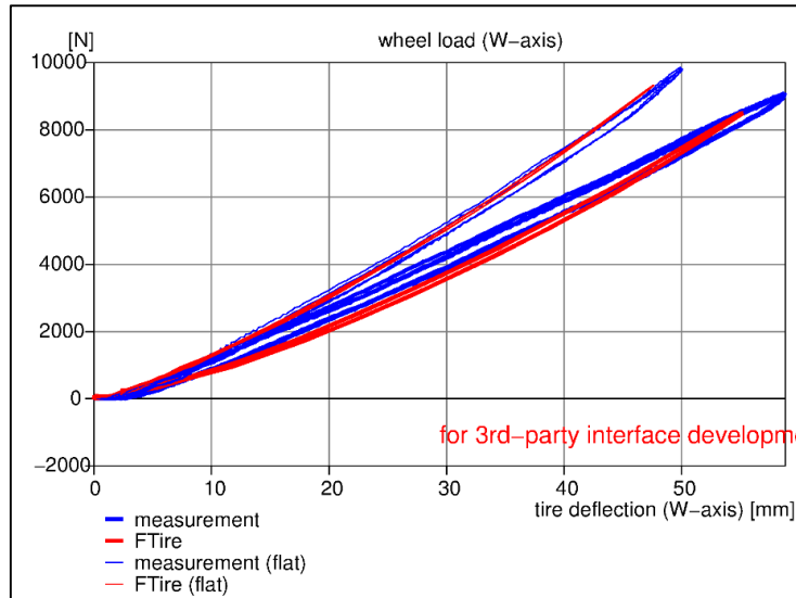
Figure 4-9: Vertical tyre stiffness on a 32x32mm transversal cleat at 0 degrees camber and 2 bar inflation pressure
