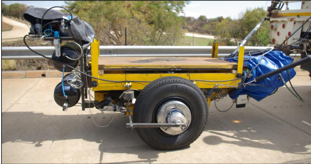
Figure 3-29: Traction validation test (LC1) at 2 bar inflation pressure
