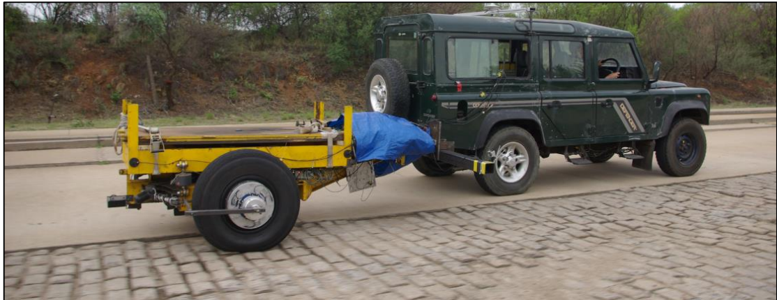
Figure 3-23: Dynamic validation test conducted on the Belgian paving
