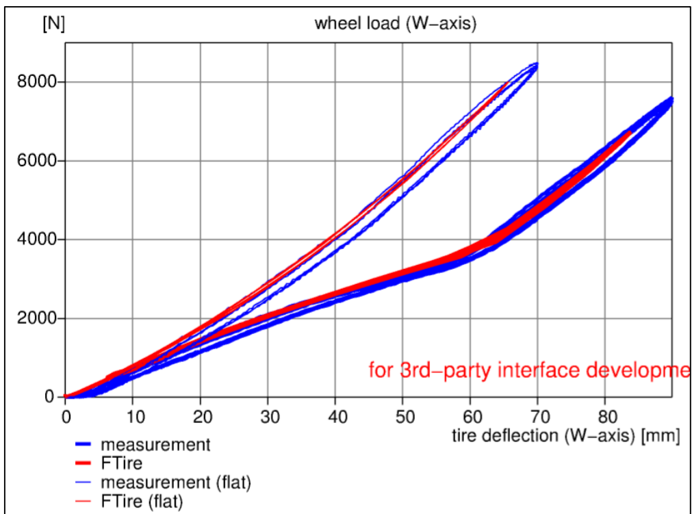
Figure 4-8: Vertical tyre stiffness on a 25x25mm transversal cleat at 0 degrees camber and 1 bar inflation pressure
