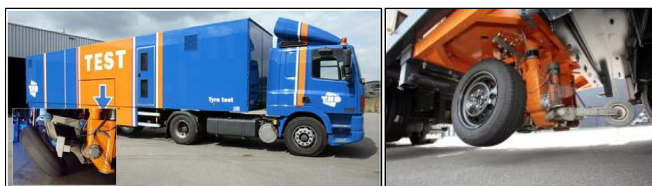
Figure 2-14: Tyre testing rig with mounted motorcycle tower (TNO, 2014)
