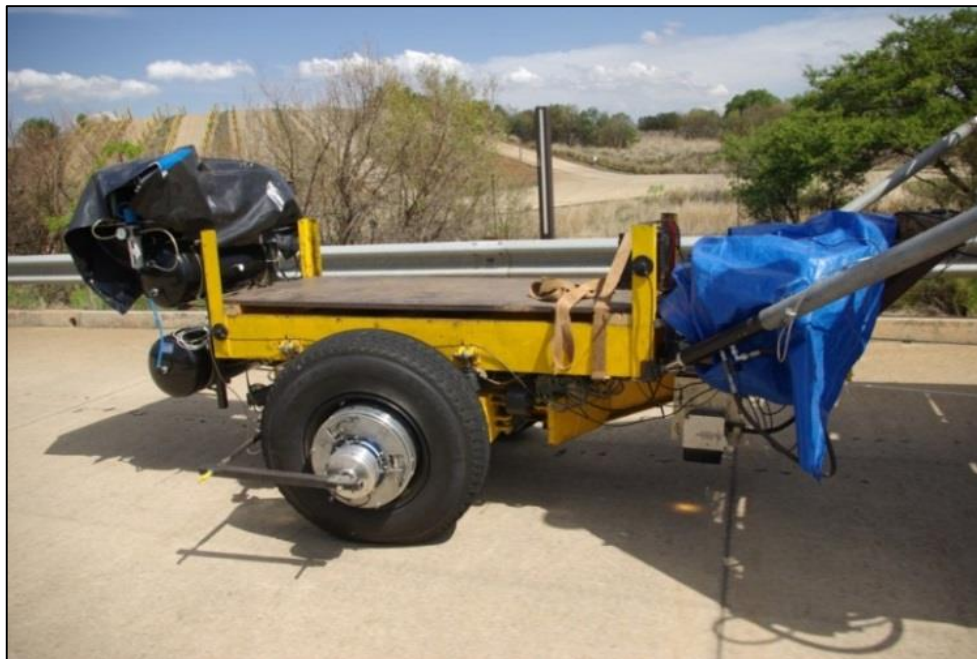
Figure 2-15: Tyre testing rig during outdoor tyre testing procedure
