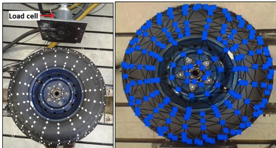
Figure 3-15: Left: Experimental setup of the modal analysis from the top. Right: Tyre, as captured by the Polytec PSV – 400 (Polytec, 2014) scanning laser vibrometer from the top
