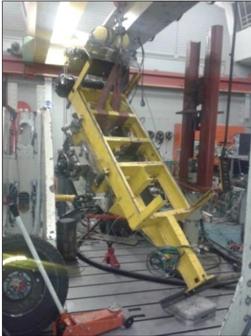
Figure 5-2: Experimental setup to determine the vertical position of the C. O. G. with pneumatic brake system
