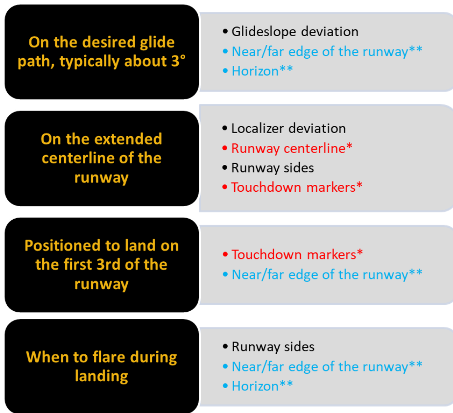
Figure 3. Visual Cues for Level 1 “Perception” Information Processing, grouped with the Level 2 Interpretations They Support [Blue (or **) indicates Cues impacted by Sensor Range, Red (or *) text indicates Cues impacted by ability to Portray Runway Markings]
