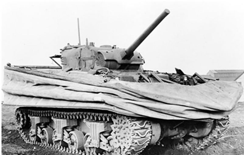
Illustration 17: DD Sherman tank with floatation screen lowered. Photo from the Imperial War Museum collection. Public domain.
