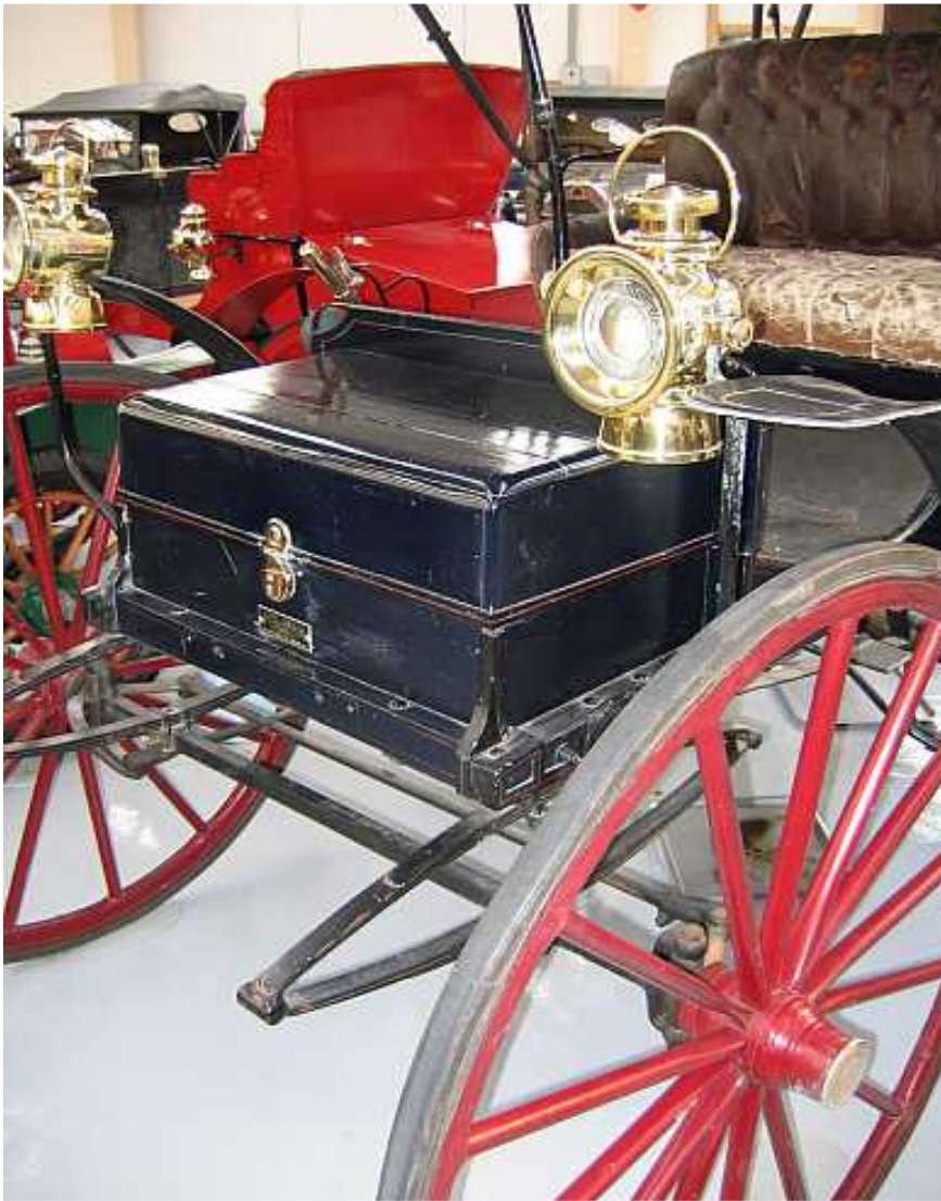
Illustration 25: Lamps and mirrors incorporated into headlights. Uni-directional forward facing illumination. Location changed to the front of the vehicle. Photo taken by the Author at the Southward Auto Museum.
