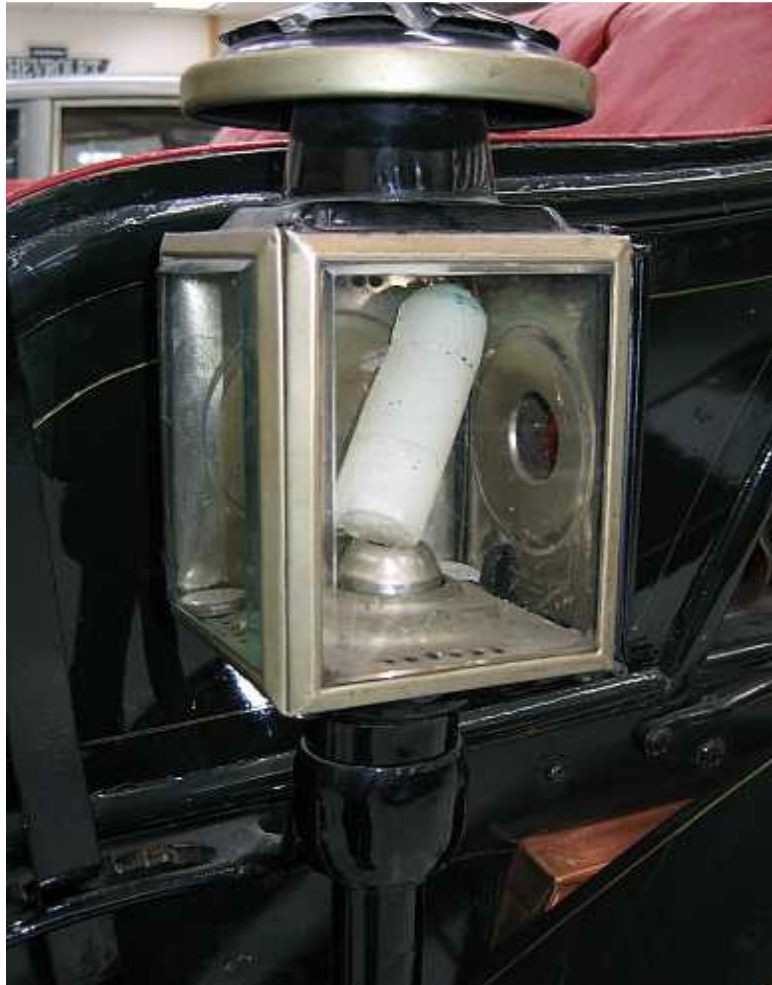
Illustration 24: Early Candle Headlight. Photo taken by the Author at the Southward Auto Museum.
