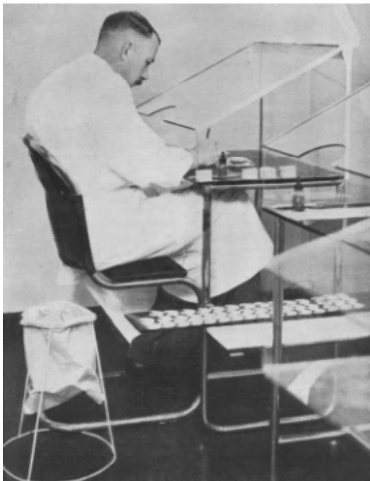
Figure 4.1: After the review of the laboratory’s safety measures, staff worked in a ventilated painting cabinet, with hard surfaces that were easy to clean. This photo is probably of J. M. C. Tingey, who led the Dominion Physical Laboratory team that used radioactive paint to illuminate dials and ammeters for military use. Source: J. M. C. Tingey, “Luminizing Army Radio Equipment”, New Zealand Journal of Science and Technology 27B (1945), p140.
