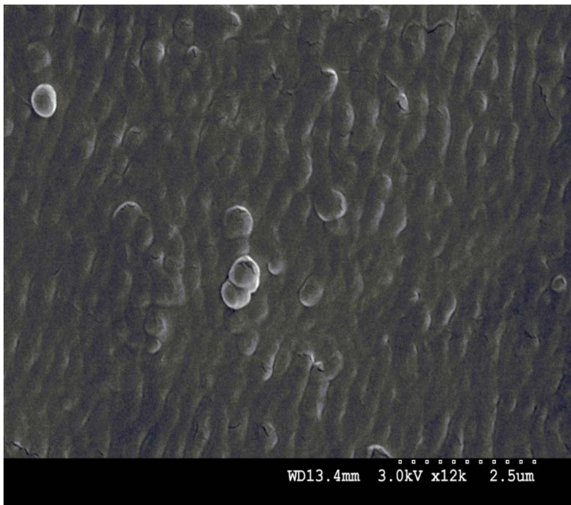
Figure 4.8. Continuous PEGMA coating formed by s-ATRP on surface PP HFM, cleaned by 36 hour extraction with acetone solvent prior to s-ATRP.
